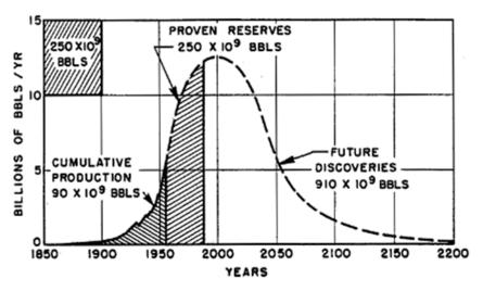
Figure 1. Ultimate global oil production (Hubbert's original calculations) [2].
