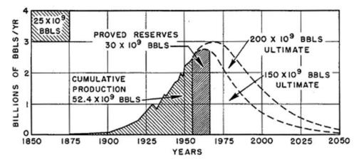
Figure 2. Ultimate US production (Hubbert's original calculations) [2].
