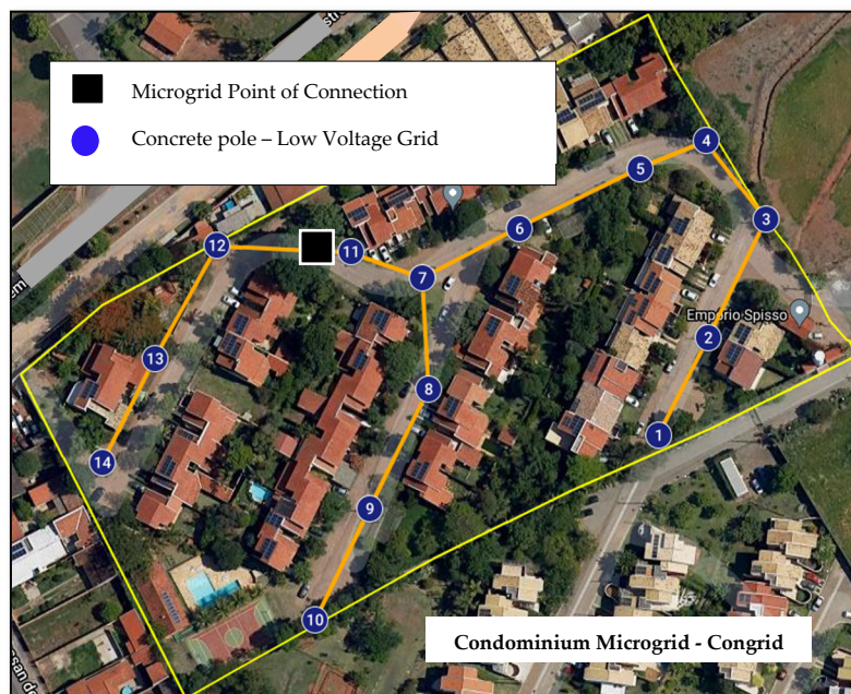
Figure 6. MERGE congrid—a condominal microgrid.
