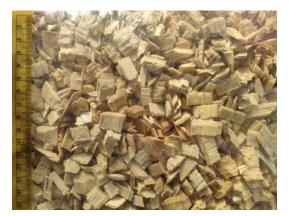
**Figure 1.** Sample of the defined wooden chips used in this study. Containing spruce with particle size of 12 to 16 mm and nearly no bark with a ruler for size comparison.
