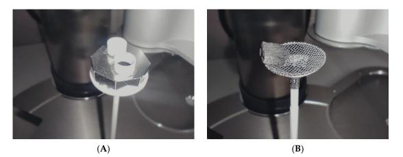
**Figure 9.** (**A**) DSC sample carrier with crucible and char powder; (**B**) TGA sample carrier with a char particle.
