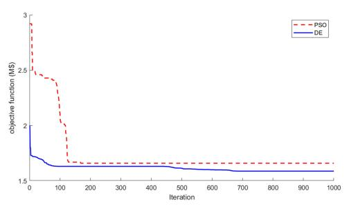
Figure 9. Convergence characteristics of the DE and PSO algorithms for case 1.
