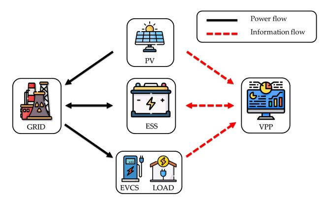
Figure 1. The structure of the VPP model.
