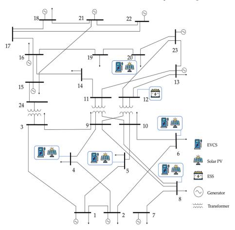
Figure 3. The RTS 24 with components of VPP.
