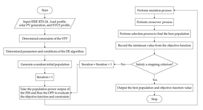
Figure 2. The proposed optimal energy management of VPP based on the DE Algorithm.
