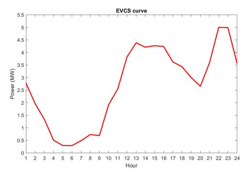
Figure 5. The typical curve of the EVCS charging profile for a day.
