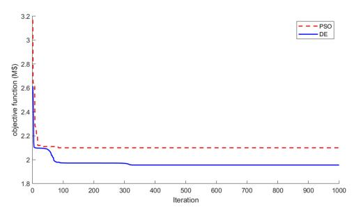
Figure 11. Convergence characteristics of the DE and PSO algorithms for case 2.
