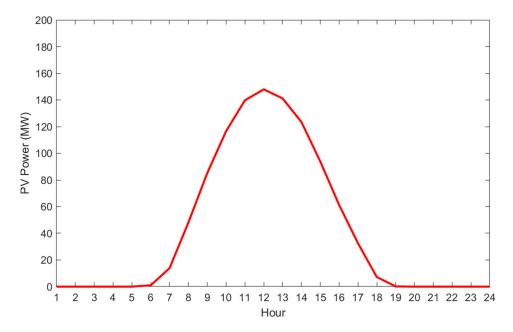
Figure 6. The daily curve of solar PV power generation.
