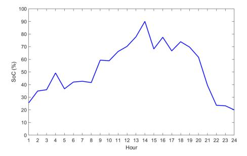
Figure 10. The SoC of ESS after solving the optimal scheduling of ESS by the DE algorithm for case 2.
