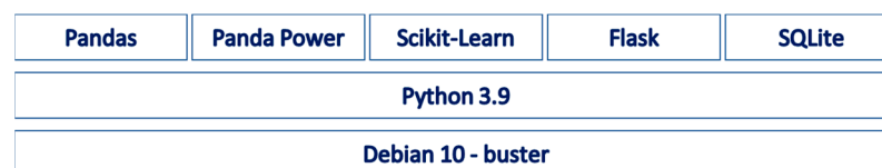
Figure 6. High-level architecture of the edge processing module software stack.
