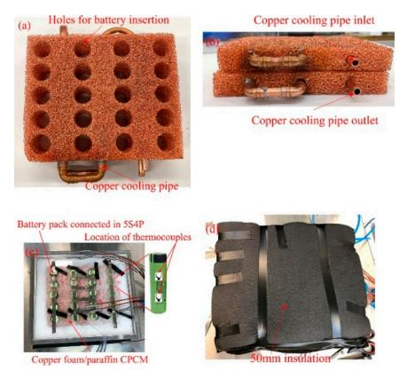
**Figure 21.** The hybrid active-passive BTMS described in [74]. (a) the Cu MF and the cooling pipes embedded into it—top view; (b) same as (a), front view; (c) PCM-impregnated Cu foam; (d) BTMS with insulation applied.
