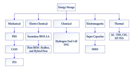
Figure 1. The hierarchical flow of energy storage systems.
