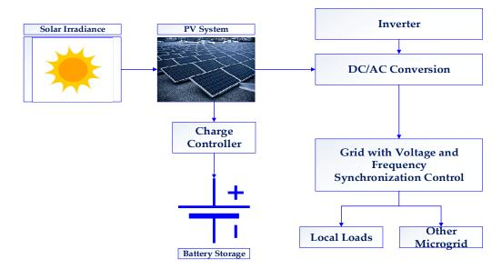
Figure 3. Schematic diagram of a DPG-ESS unit.
