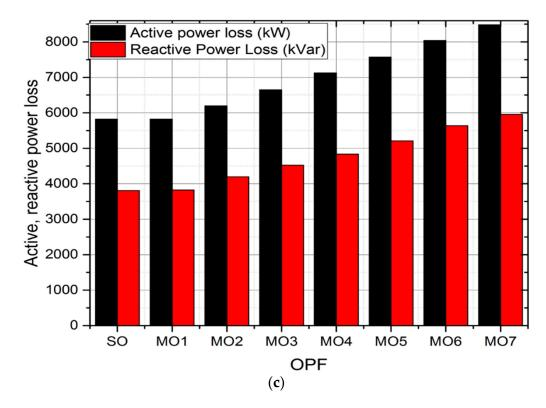
**Figure 7.** (**a**) The cost is related to different objectives. (**b**) Cost saving and voltage index for OPF. (**c**) Reactive and accurate PL profile.
