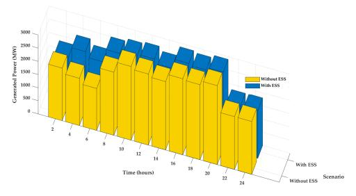
Figure 6. Load leveling features in the presence and absence of ESS.
