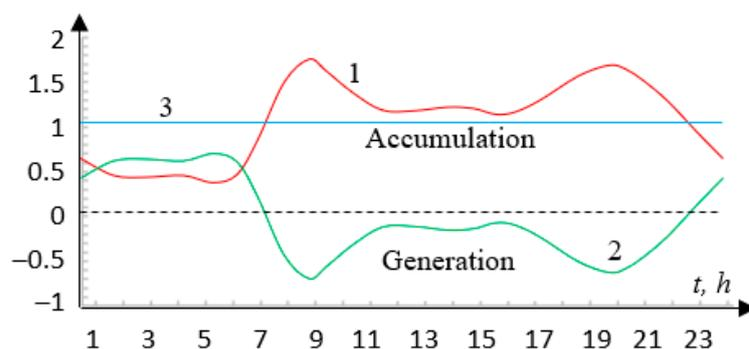
**Figure 1.** Dependence graphs for normalized capacities: 1—graph of the electricity consumption function  $P_{p.nor}(t)$ ; 2—graph of the function for ESS  $P_{p.nor}(t)$ ; 3—the graph of the function of the sum of the powers of all generators  $P_{g.nor}(t) = 1$ .
