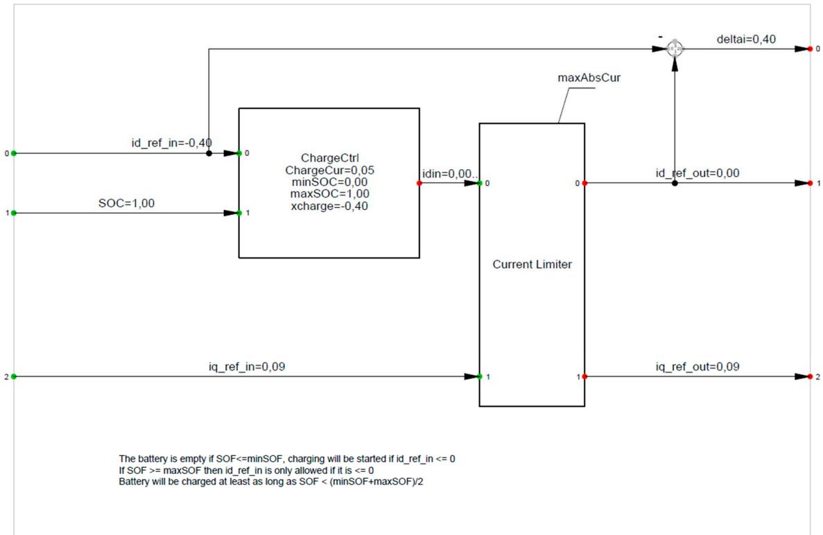
Figure 4. Model of charge–discharge regulator.
