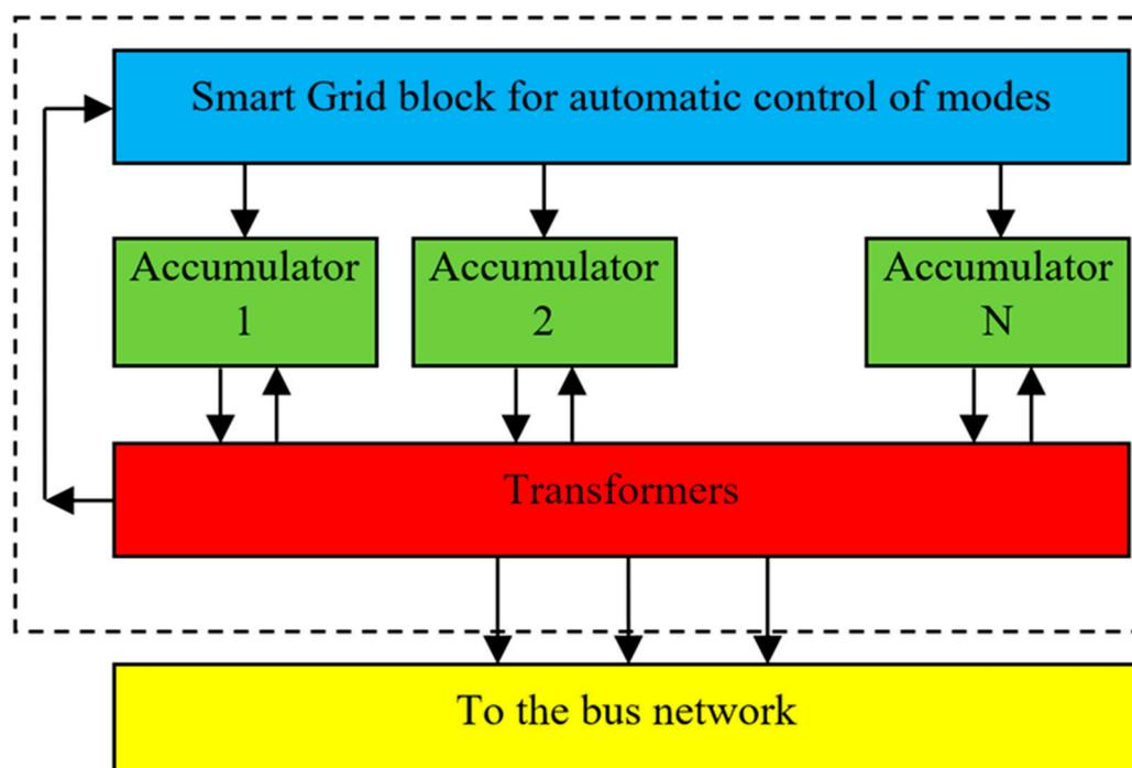
**Figure 2.** Structural diagram of Smart Grid with electricity storage system.
