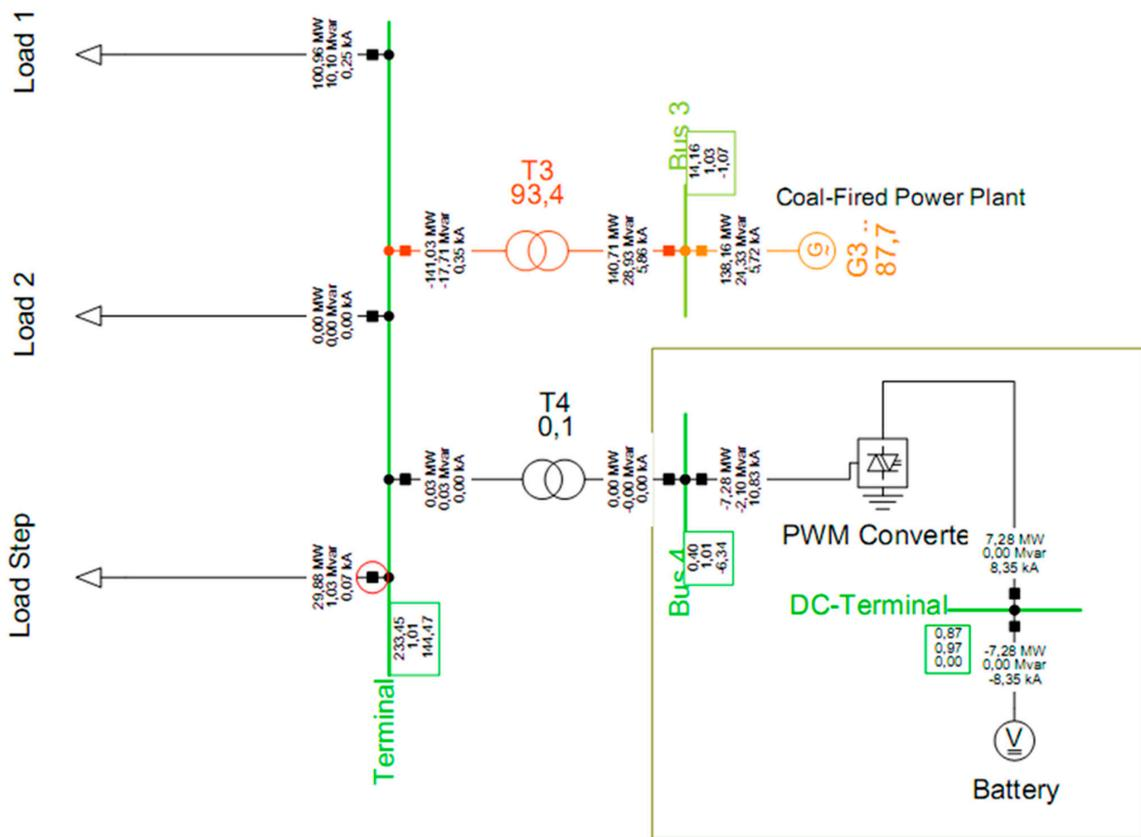
Figure 3. Test network for testing ESS.
