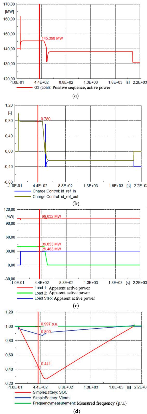
**Figure 5.** The results of test studies of the SNE when the network load changes. (a) Active load schedule of generator G3, taking into account the influence of the ESS. (b) ESS battery charge charts. (c) Timing diagram for load initiation and end in the network. (d) Change in the capacity and voltage of the ESS batteries over time.
