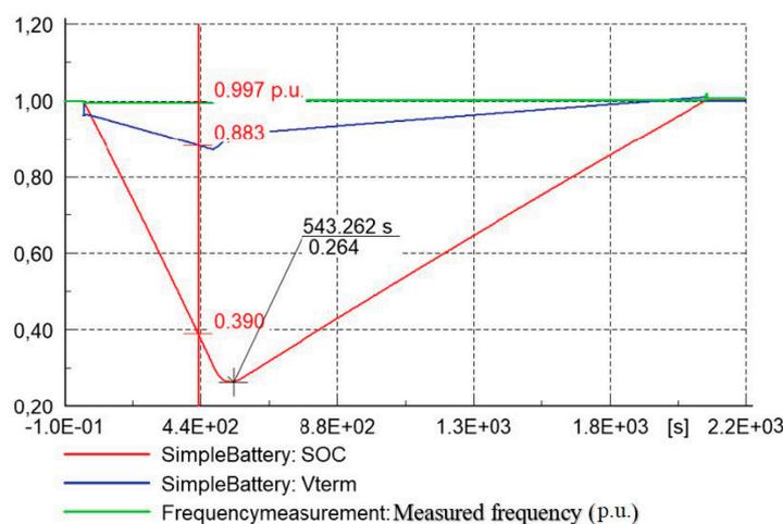
**Figure 6.** Results of simulation of discharge and charge of ESS.
