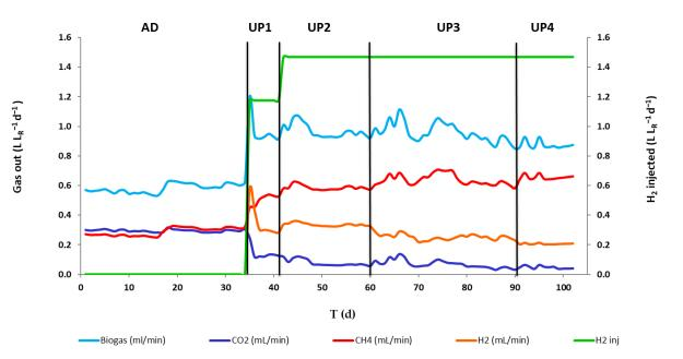
Figure 1. Daily time courses of biogas H<sub>2</sub>, CH<sub>4</sub>, CO<sub>2</sub> flow rates of all experimental phases.
