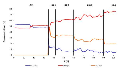
Figure 2. Biogas composition: H<sub>2</sub>, CH<sub>4</sub>, CO<sub>2</sub> (%), during all experimental phases.
