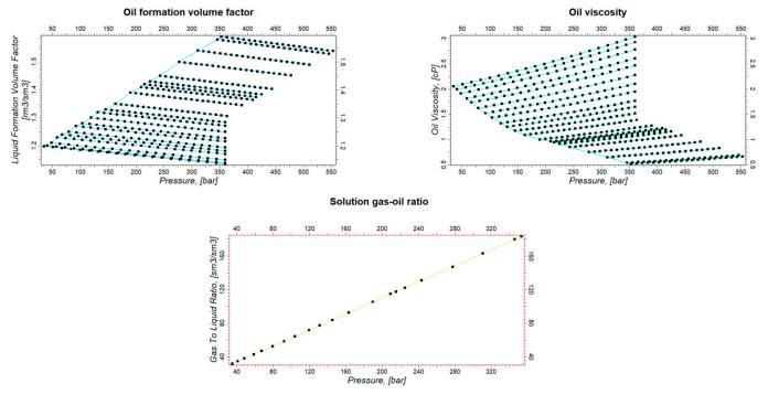
the initialization of the oil phase, the dissolved gas and the water phase. Figure 6 shows the oil properties and Figure 7 demonstrates the gas properties used in the model.
