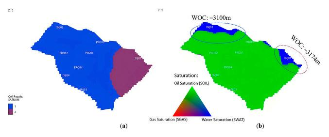
**Figure 10.** Water-oil contact (WOC) definition: (**a**) Region definition (**b**) Distribution of initial fluid saturation.
