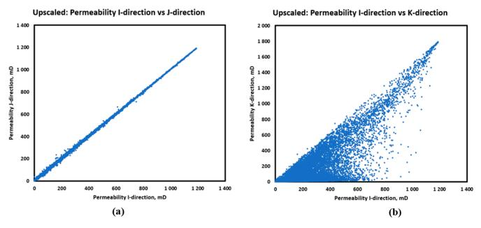
Figure 4. Upscaled permeability relationship in: (a) I-J direction; (b) I-K direction.
