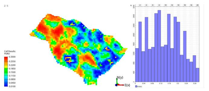
Figure 2. UNISIM-I-D upscaled porosity results.
