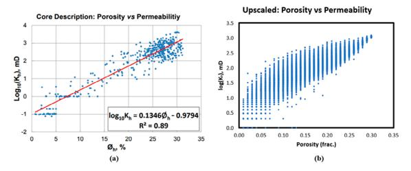
**Figure 3.** Porosity versus permeability: (**a**) Core analysis data [19] in which the blue dot refers to the core sample whereas the red line refers to the equation and (**b**) Upscaled model.
