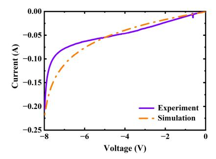
Figure 10. Polarization curves obtained through experiment and simulation.
