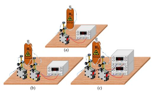
Figure 1. Experimental equipment: (a) SC–SP, (b) DC–SP, and (c) DC–DP systems.
