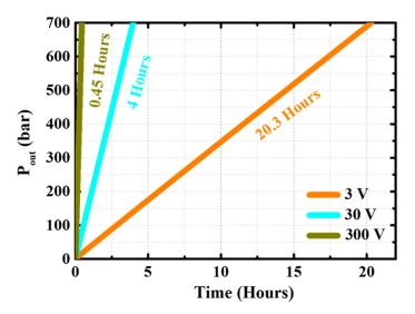
Figure 12. Time required to reach a pressure of 700 bar at different voltages.
