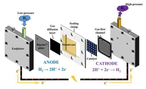
Figure 2. EHC design and principle.
