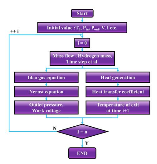
Figure 3. Flow chart of the analytical model.
