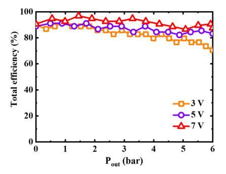
**Figure 11.** Compression efficiency when the anode pressure was 1 bar and the applied voltage was 3, 5, and 7 V.
