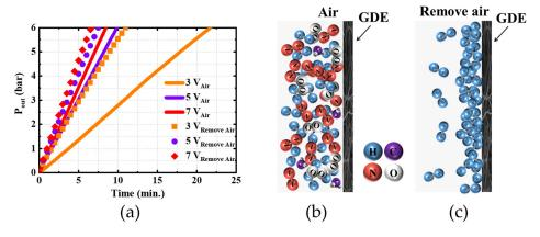
**Figure 4.** (a) Effect of the presence or absence of air in the anode on the cathode pressure at an inlet pressure of 1 bar. (b) Anode chamber without air removed. (c) Anode chamber with air removed.
