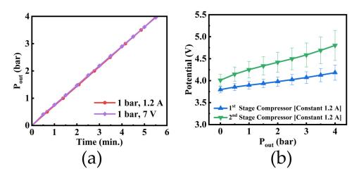
**Figure 6.** The DC–DP system, applying a constant current and voltage at an anode pressure of 1 bar. (a) Compression rate when a constant current or constant voltage is applied. (b) Voltage changes as a function of the cathode pressure when a constant current is applied.
