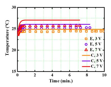
Figure 9. Comparison of the experimental and simulation results on the cathode temperature.
