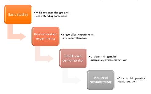
Figure 11. The four-step process proposed for the development of a breakthrough reactor system.
