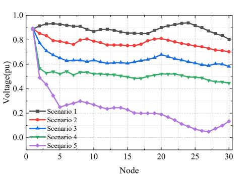
Figure 4. Unit value of node voltage under different distributed generation penetration rates.
