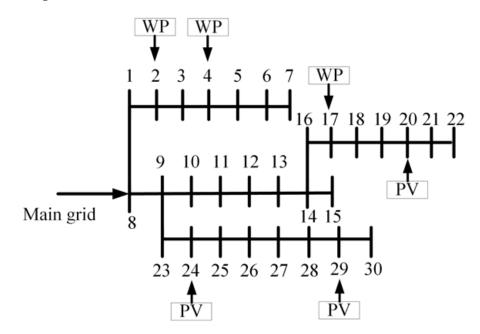
Figure 1. Improved IEEE 30 node distribution network system structure diagram.
