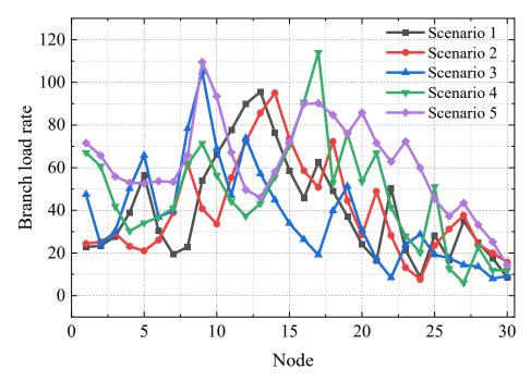
Figure 5. Branch load rate under different distributed power penetration.
