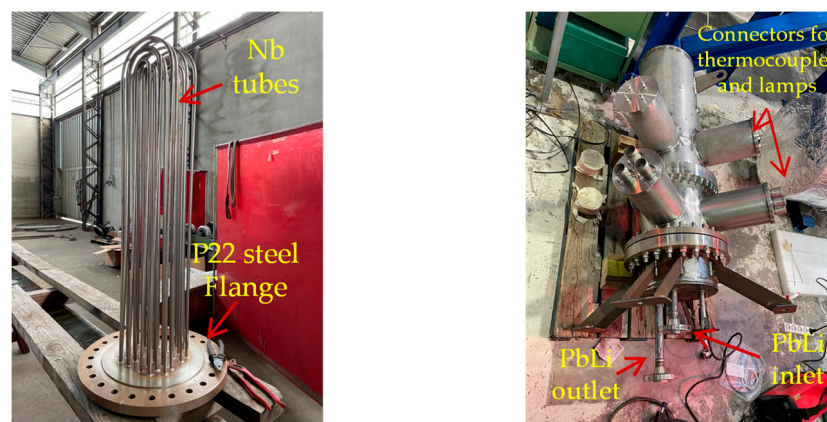
Figure 2. Pictures of the PAV mock-up at the end of the manufacturing.
