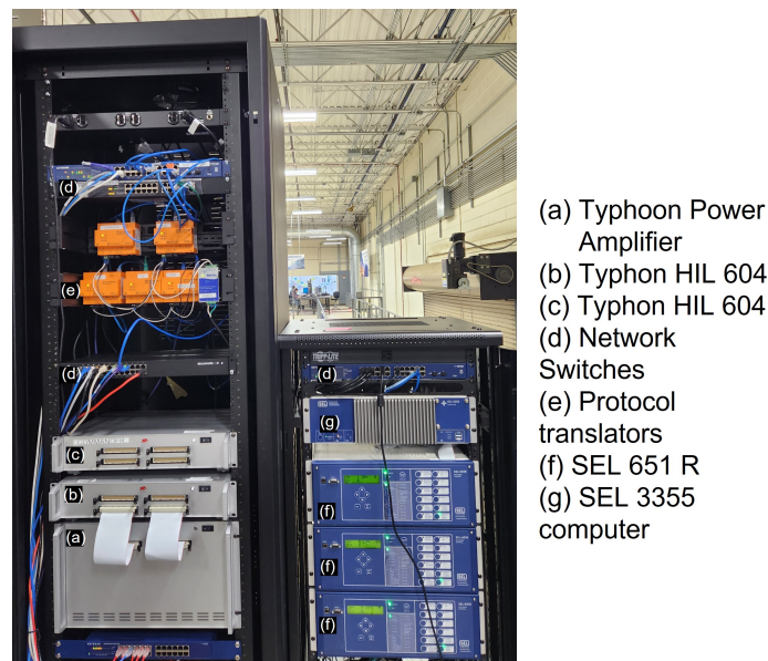
Figure 18. The HIL test bed of Adjuntas 2-microgrid system.
