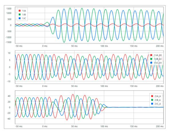
**Figure 6.** F2 line-to-line fault event traces: CB2 relay currents (**top** chart) in A, CB2 relay 11 kV line-to-ground voltages (**middle** chart) in kV, and CB21 relay currents (**bottom** chart) in A.
