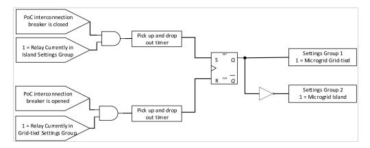
**Figure 3.** An example, simplified protection logic using the Control System Countermeasures method.
