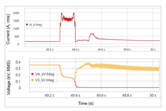
**Figure 5.** Point of Connection (PoC) current magnitude (**top** chart), utility voltage magnitude (**bottom** chart: red trace), and microgrid voltage magnitude (**bottom** chart: yellow trace).
