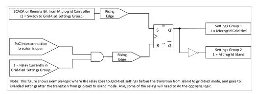
Figure 2. An example, simplified logic using the Microgrid Adaptive Relaying method.
