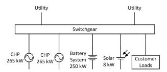
Figure 4. Example Microgrid #1—simplified single line diagram.
