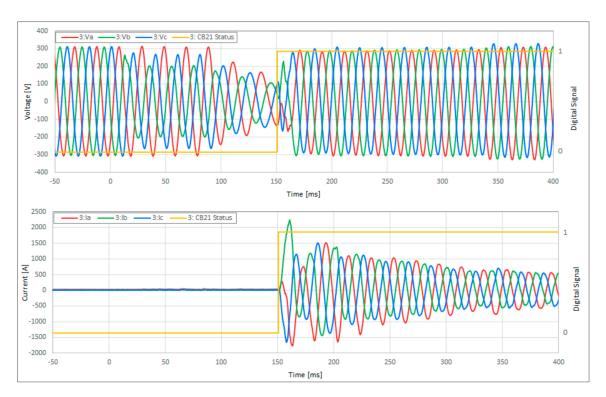
**Figure 7.** F2 line-to-line fault event traces: one of two Battery Energy Storage System (BESS) inverter terminal voltages (**top** chart) and terminal currents of the same BESS inverter (**bottom** chart).
