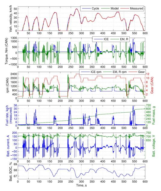
**Figure 6.** Example of CiL testing results simulating the hybrid powertrain operation in a driving cycle.
