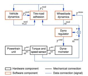
**Figure 2.** Hardware arrangement, simulation and control loops of a CiL system for powertrain testing with a vehicle model taking into account the tire slip.
