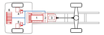
**Figure 3.** The studied hybrid powertrain intended for a heavy-duty vehicle. 1—internal combustion engine, 2—hybrid module, 3—automated gearbox, 4, 5—front electric drives with reduction gears, 6—traction battery.
