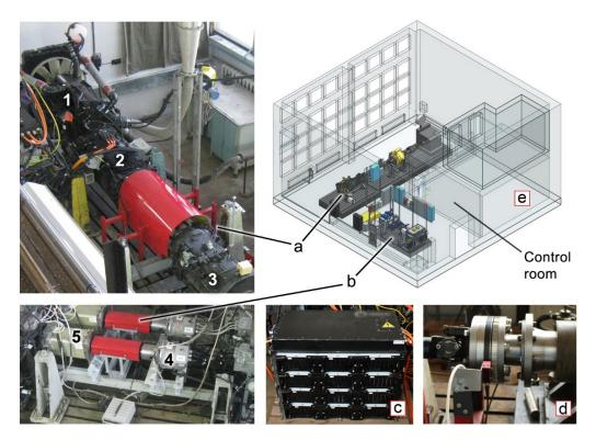
**Figure 5.** Laboratory setup for CiL testing of the hybrid powertrain. **a**—test bench for the rear driveline, **b**—test bench for the front electric drives, **c**—traction battery, **d**—torque and rpm sensor installed in the rear driveline's test bench, **e**—CAD model of the testing facility. 1—engine, 2— automated gearbox with the hybrid module, 3—loading gearbox, 4—front electric drive, 5—front loading device.
