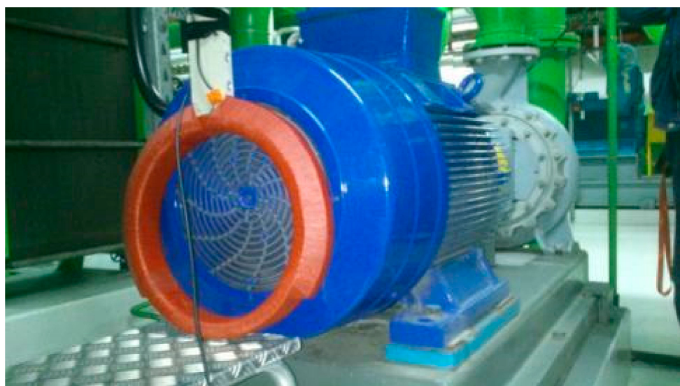
Figure 18. Flux measurement coil located on the non-driving side of the motor.
