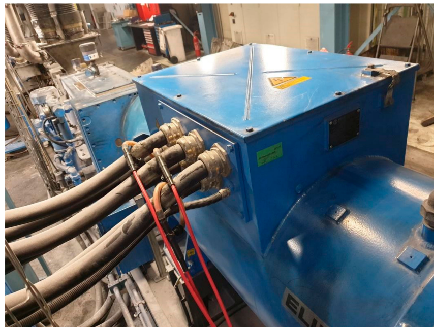
Figure 14. Direct measurement of the motor phase currents with use of Rogowski coils.
