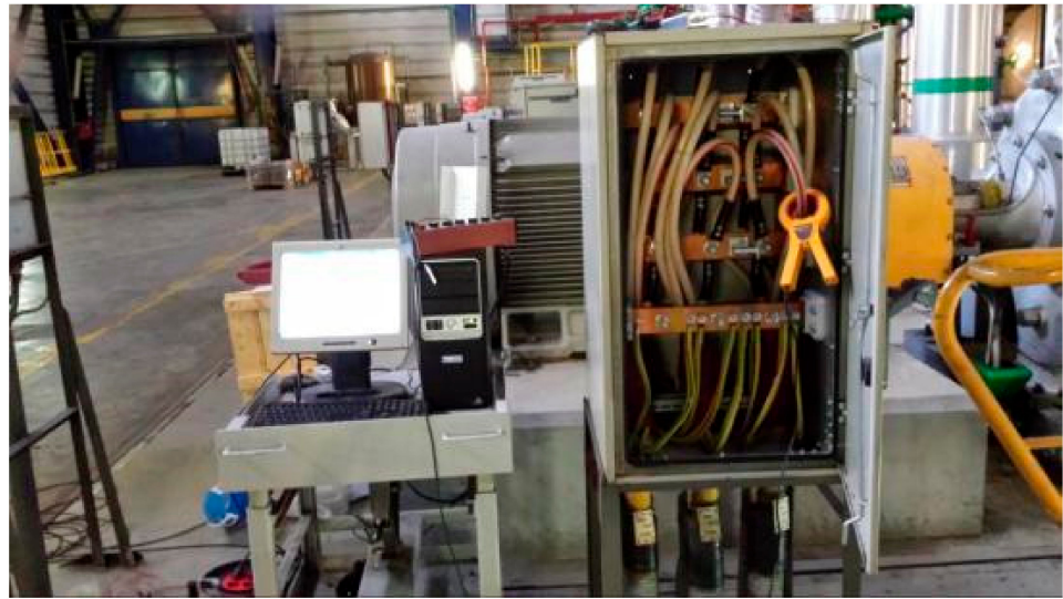
Figure 15. Direct measurement of one phase current at the output of the inverter.
