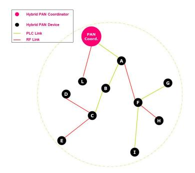
Figure 15. Typical hybrid network topology.
