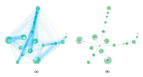
Figure 6. Links (a) and routes (b) over a same G3-PLC network topology.
