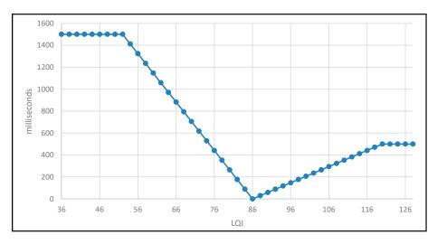
Figure 9. Representation of the jittering delay as a function of the LQI.
