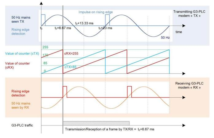
Figure 5. G3-PLC phase detection principle.
