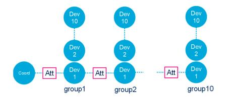
Figure 10. Network topology for testing the RREQ jittering mechanism.
