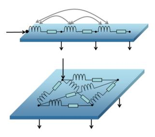
**Figure 9.** Electrical representation of conductors linking more than two points. **(Top)**, the current path is quite obvious, and an electrical representation can be "guessed". **(Bottom)**, the case of a plate with no straightforward representation, except for the "heavy" full connection of each point with R-L coupled elements (mutual coupling not displayed for clarity).
