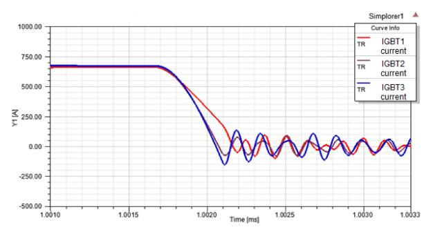
**Figure 7.** Simulated results of current division among the three bottom switches of phase W with power layout only, identical idealized gate signals.
