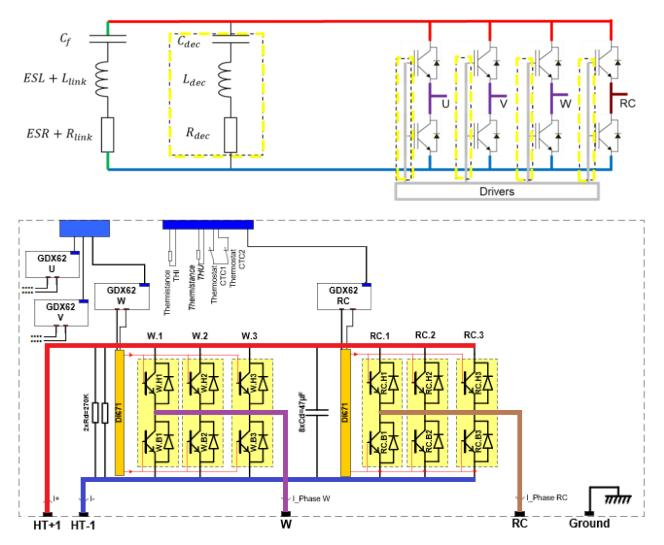
**Figure 1.** Railway inverter composition. The global function is a three-phase inverter with one additional non-reversible leg for braking. Each leg uses three paralleled IGBT modules. The full converter is built from two identical subparts composed of two legs and decoupling capacitors (bottom of the figure). A common DC capacitor tank is used to provide the energy storage at DC-bus level.
