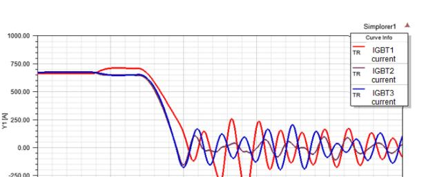
**Figure 8.** Simulated results of current divisions among the three bottom switches of phase W with power layout and Gate Distribution PCB layout—no coupling considered.
