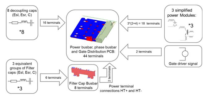
**Figure 5.** Time domain simulation scheme. Two Partial Element Equivalent Circuit (PEEC) models used from separate files: power and phase busbar plus Gate Distribution PCB and DC capacitor tank busbar. Equivalent esr–esl models of the decoupling capacitors and the three blocks of the DC Capacitor tank. "Home made" IGBT and diode models are used. Idealized drive signal is a simple voltage source.
