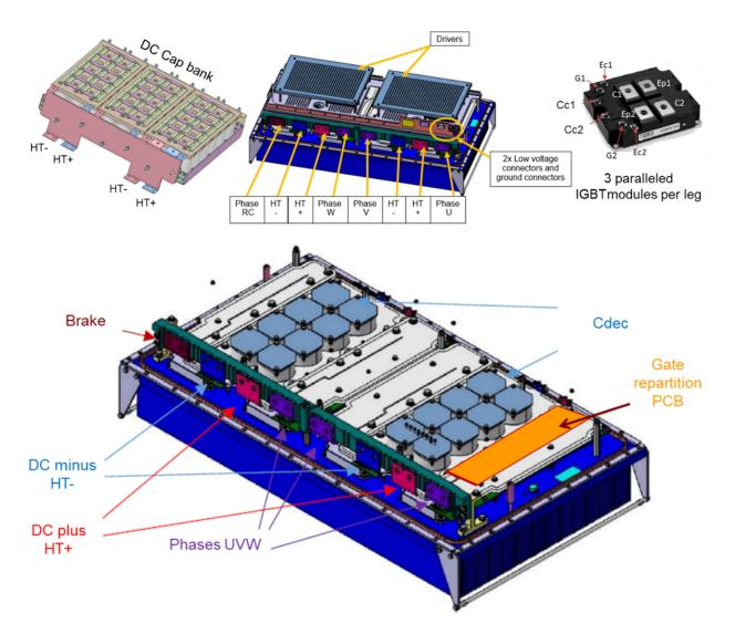
**Figure 2.** (**Top: left**), DC capacitor bank with duplicated DC bus connections, one for each subpart. (**Center**), overview of the global 3D layout. (**Right**), IGBT power Module. (**Bottom**): 3D layout of the power part.
