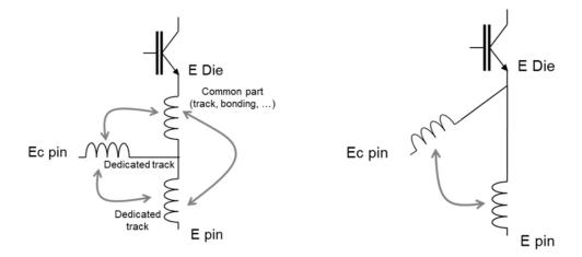
**Figure 13.** Example of a PEEC representation in the case of classical common emitter coupling. The (**left**) representation is based on the geometry and the proposed generic representation; (**right**) is based on terminals only and is independent from the geometry. Both account for exactly the same phenomena.
