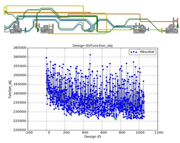
**Figure 17. (Top**): Optimized Gate Distribution PCB corresponding to the optimal point. (**Bottom**): evolution of the objective function vs iterations. The green point corresponds to the minimum of the objective function.
