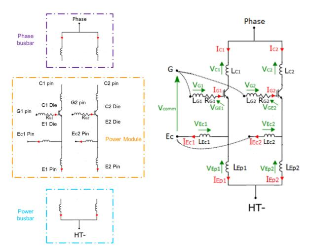
Figure 12. (Left): individual models of each part of the system. (Right): reduction of the model by associating series elements.
