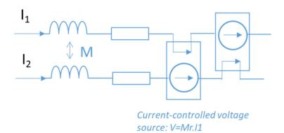
Figure 11. A possible way to reproduce "resistive couplings" in Pspice-compatible representations.
