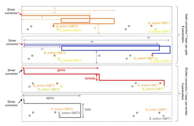
Figure 16. Gate Distribution PCB: parametrized geometry.
