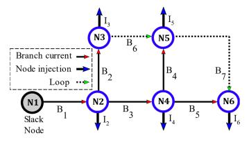
Figure 1. Graph of a simple low voltage direct current (LVDC) distribution system.
