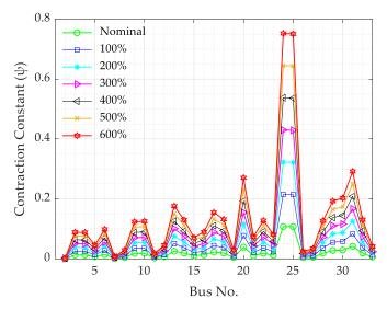
Figure 14. Value of the contraction constant for each node (33-node) for different loading conditions.
