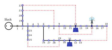
Figure 2. Modified 33-node LVDC test feeder [3,4].
