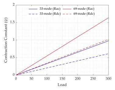
Figure 13. Maximum allowable loading with R<sub>ac</sub> and R<sub>dc</sub> in terms of a contraction constant.
