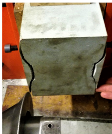
Figure 10. A view of the sandstone block after the mining with disk tools 150 mm in diameter and edge angle 40^\circ .
