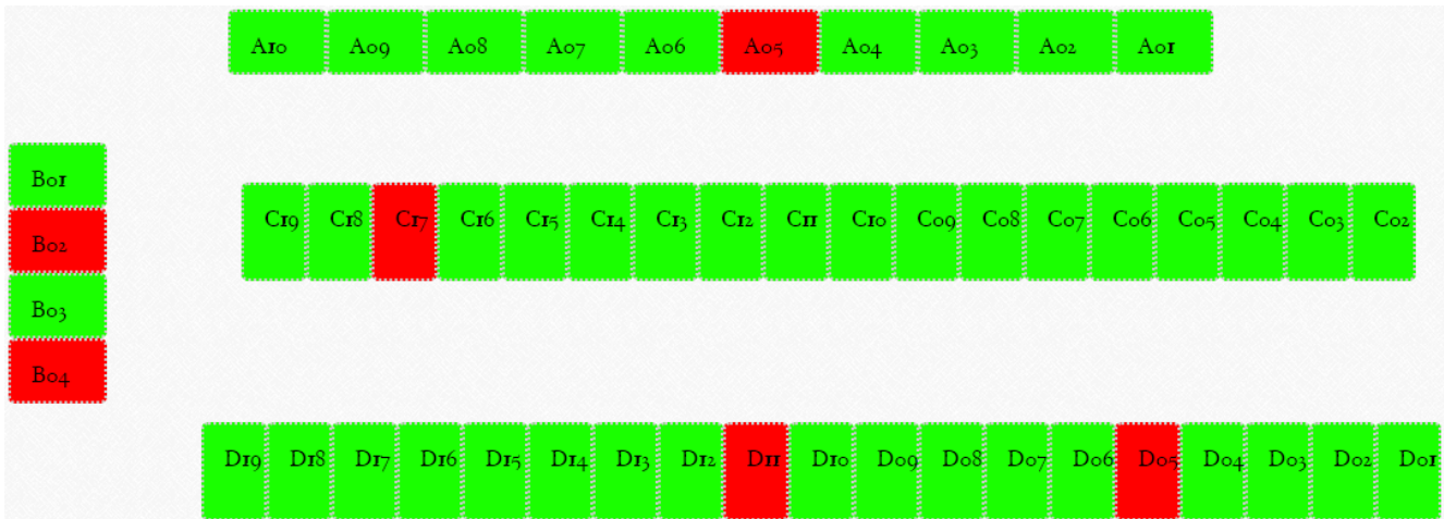
Figure 15. Parking Status: Red for occupied spots and green for vacant ones.
