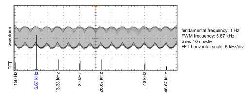
**Figure 6.** Oscillogram of the earth fault current in a variable-speed drive circuit (earth fault at the motor terminals). The motor is supplied by frequency 1 Hz (very slow motor speed); pulse width modulation (PWM) frequency: 6.67 kHz.
