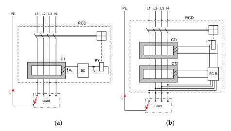
**Figure 1.** Structure of residual current devices (RCDs): (a) voltage-independent (AC-type, A-type, F-type); (b) voltage-dependent (B-type); RCD—residual current device; CT, CT1, CT2—current transformers; EC—electronic matching system (e.g., to increase the sensitivity to the DC pulsating waveform); EC-B—electronic system which ensures tripping especially in the case of the smooth DC residual current; RY—relay.
