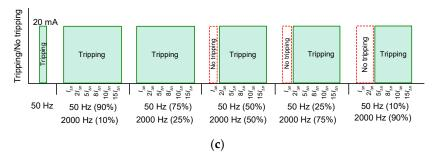
**Figure 11.** Tripping of the 30 mA F-type RCD (no. RCD\_1F—symbol defined in Table 2) for waveform composed of the fundamental frequency (50 Hz) and high-frequency component: (a) 500 Hz; (b) 1000 Hz; (c) 2000 Hz. Values in brackets indicate the content of the particular component; 20 mA—real tripping current for a pure sinusoidal signal of 50 Hz.
