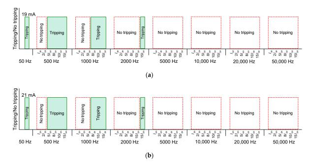
**Figure 16.** Tripping of the 30 mA B-type RCDs for a sine waveform of the specified frequency from 50 Hz to 50 kHz: (a) RCD\_1B; (b) RCD\_2B; symbols defined in Table 2.
