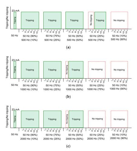
**Figure 10.** Tripping of the 30 mA A-type RCD (no. RCD\_1A—symbol defined in Table 2) for waveform composed of the fundamental frequency (50 Hz) and high-frequency component: (a) 500 Hz; (b) 1000 Hz; (c) 2000 Hz. Values in brackets indicate the content of the particular component; 23 mA—real tripping current for a pure sinusoidal signal of 50 Hz.
