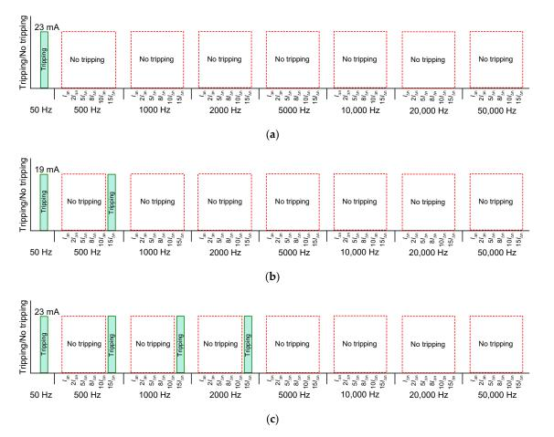
**Figure 14.** Tripping of the 30 mA A-type RCDs for a sine waveform of the specified frequency from 50 Hz to 50 kHz: (a) RCD\_1A; (b) RCD\_2A; (c) RCD\_3A; symbols defined in Table 2.
