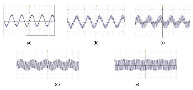
**Figure 8.** Example waveforms (time: 10 ms/div) composed of two frequencies, generated by the laboratory generator: (a) 50 Hz (90%) and 1000 Hz (10%); (b) 50 Hz (75%) and 1000 Hz (25%); (c) 50 Hz (50%) and 1000 Hz (50%); (d) 50 Hz (25%) and 1000 Hz (75%); (e) 50 Hz (10%) and 1000 Hz (90%).
