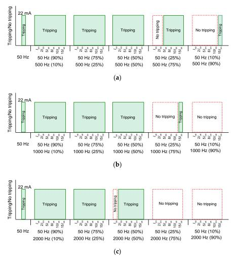
**Figure 9.** Tripping of the 30 mA AC-type RCD (no. RCD\_1AC—symbol defined in Table 2) for waveform composed of the fundamental frequency (50 Hz) and high-frequency component: (a) 500 Hz; (b) 1000 Hz; (c) 2000 Hz. Values in brackets indicate the content of the particular component; 22 mA—real tripping current for a pure sinusoidal signal of 50 Hz.
