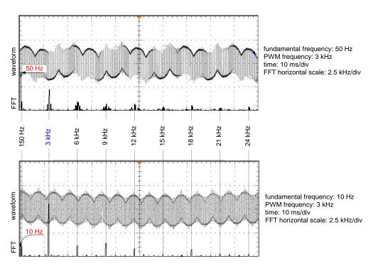
**Figure 5.** Oscillograms of the earth fault current in a variable-speed drive circuit (earth fault at the motor terminals). Upper oscillogram: the motor is supplied by frequency 50 Hz (rated motor speed); lower oscillogram: the motor is supplied by frequency 10 Hz (slow motor speed); pulse width modulation (PWM) frequency: 3 kHz.
