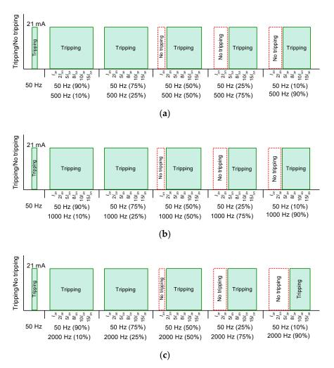
**Figure 12.** Tripping of the 30 mA B-type RCD (no. RCD\_2B—symbol defined in Table 2) for waveform composed of the fundamental frequency (50 Hz) and high-frequency component: (a) 500 Hz; (b) 1000 Hz; (c) 2000 Hz. Values in brackets indicate the content of the particular component; 21 mA—real tripping current for a pure sinusoidal signal of 50 Hz.
