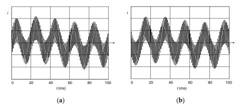
**Figure 3.** Mixed-frequency waveform composed of components presented in Table 1; phase angle of the  $I_{1\text{kHz}}$  and  $I_{10\text{Hz}}$  is  $0^{\circ}$ ; phase angle of the  $I_{\text{fund}}$  (50 Hz) is: (a)  $0^{\circ}$ ; (b)  $180^{\circ}$ .
