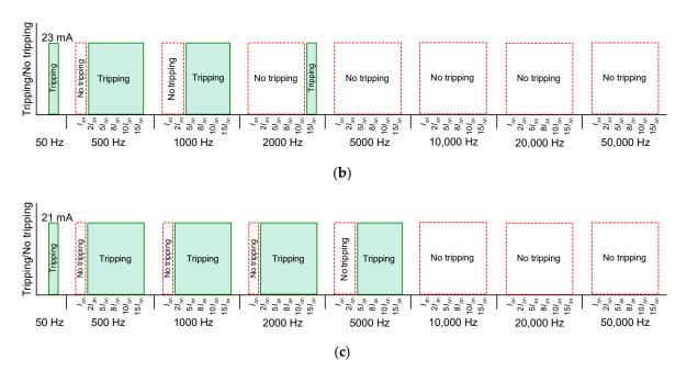
**Figure 13.** Tripping of the 30 mA AC-type RCDs for a sine waveform of the specified frequency from 50 Hz to 50 kHz: (a) RCD\_1AC; (b) RCD\_2AC; (c) RCD\_3AC; symbols defined in Table 2.
