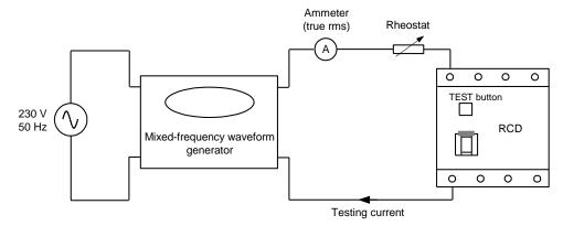
Figure 7. Laboratory stand for RCDs testing.
