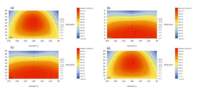
**Figure 6.** The intensity of solar radiation depending on the Photovoltaic panel tilt angle in each season: (**a**) optimal tilt 49.5 receiving 519 kWh/m<sup>2</sup> during winter; (**b**) optimal tilt 13.5 receiving 669.22 kWh/m<sup>2</sup> during spring; (**c**) optimal tilt 13.5 receiving 689 kWh/m<sup>2</sup> during summer; (**d**) optimal tilt 49.5 receiving 498 kWh/m<sup>2</sup> during the autumn.
