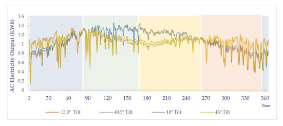
Figure 7. Impact of the tilt angle on the PV panel's electricity Output in each season.
