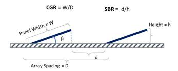
**Figure 2.** Profile view of Photovoltaic system layout on a flat roof illustrating the *CGR* (Coverage Ground Ratio) and *SBR* (Setback Ratio) [47], adapted.
