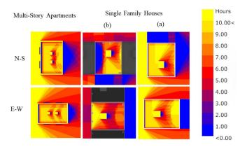
Figure 5. Shadows mesh on residential typologies roofs on solstice winter.
