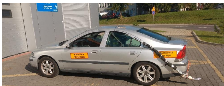
Figure 4. View of the tested vehicle with the portable emission measurement system (PEMS) system.
