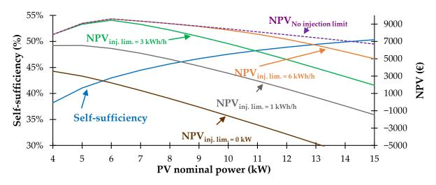
Figure 11. Self-sufficiency and NET Present Value (NPV) as functions of PV nominal power with different injection limits.
