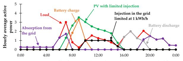
Figure 13. Hourly energy profiles of Figure 11 with a curtailment in the grid injection *I.L.* = 1 kWh/h.
