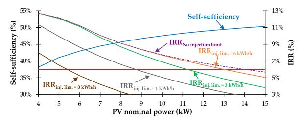
Figure 9. Self-sufficiency and IRR as functions of PV nominal power for different injection limits.
