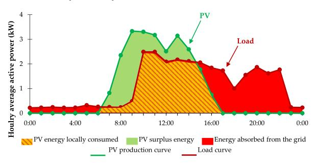
Figure 1. Generic example of PV generation and load profiles of a domestic user.
