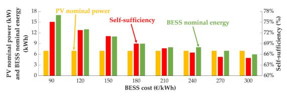
Figure 14. PV nominal power, BESS nominal energy, and maximum SS for different BESS costs.
