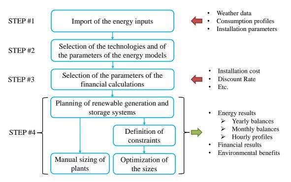
Figure 2. Scheme of the procedure used in the tool with indication of the inputs/outputs.
