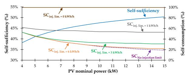
Figure 10. SC and SS as functions of PV nominal power with different injection limits.
