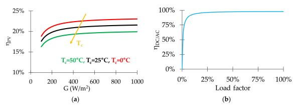
Figure 4. PV efficiency as function of irradiance and temperature (a) and DC/AC conversion efficiency (b).
