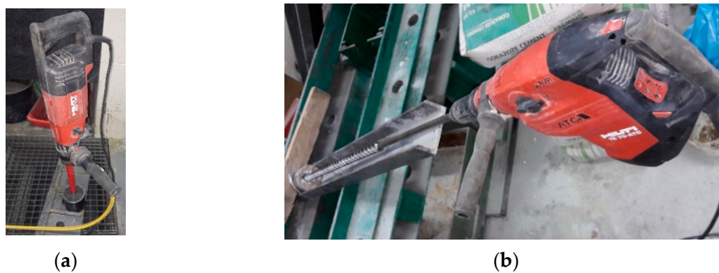
Figure 5. Drilling holes with application: (a) Crown drill; (b) Hammer drill bit with SDS MAX mounting.
