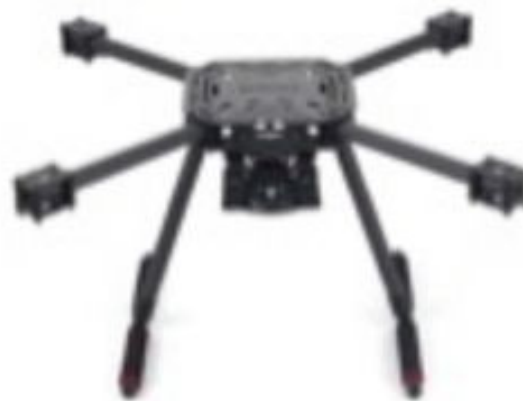
Figure 6. Quadcopter 500 mm Carbon Fibre frame of the 5G-enabled UAV prototype.
