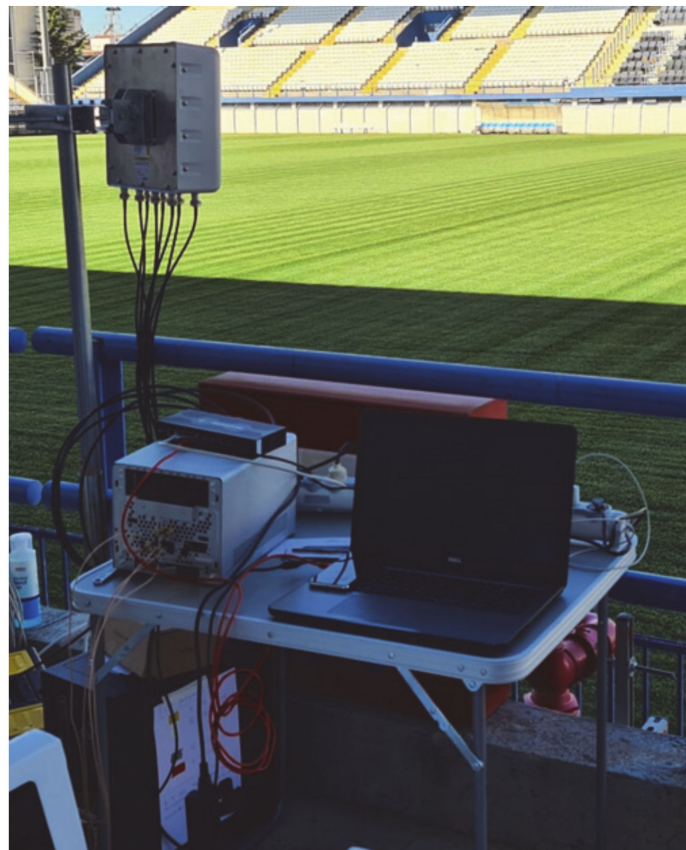
Figure 3. 5G Infrastructure deployed in field for executing feasibility trials of 5G-enable and energy efficient UAV.
