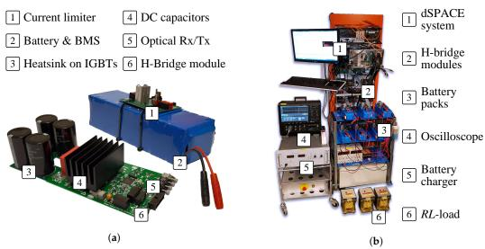
**Figure 16.** (a) H-bridge module with 48 V battery pack; (b) Small-scale CHB inverter setup, including battery packs, with control and measurement equipment.
