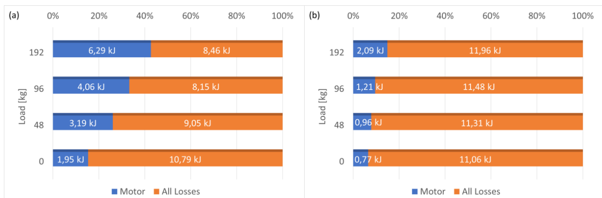
Figure 8. Motor vs. all losses: (a) conventional drive, (b) EHD.
