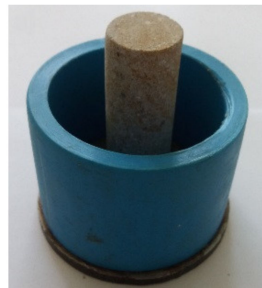
Figure 8. Sandstone core ready to be sealed with cement slurry.
