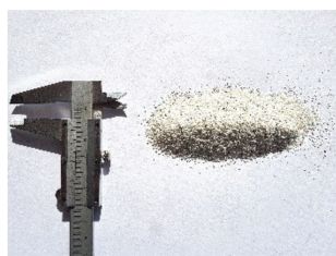
Figure 2. Medium-weight coarse-grained abrasive fraction.
