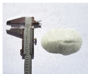
Figure 3. Fine-grained abrasive fraction to improve the hydraulic parameters of the liquid.
