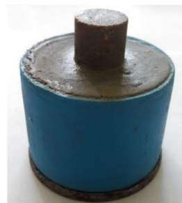
Figure 9. Sandstone core ready for adhesion testing on contact with cement slurry.
