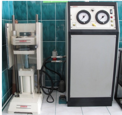
Figure 10. Device for measuring adhesion on the contact of tested surfaces.
