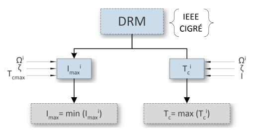
Figure 1. Dynamic Rating Management (DRM) system flowchart.
