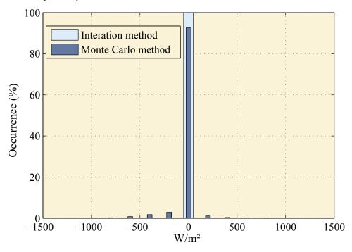
Figure 18. Differences between measured and effective solar radiation.
