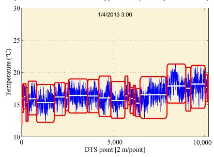
Figure 10. Evolution of conductor temperature along the line in a specific date.
