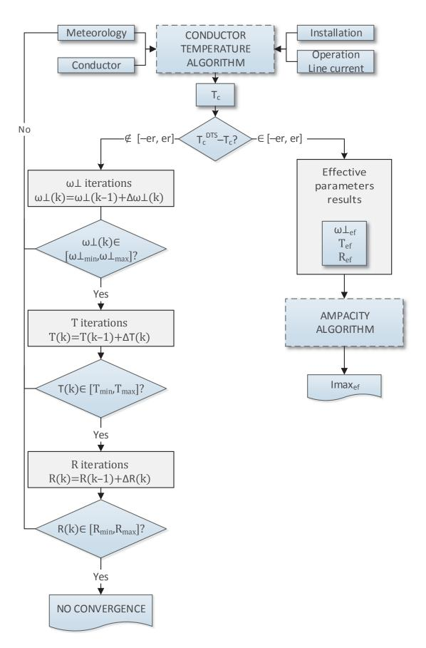
Figure 11. Iteration method flow diagram.
