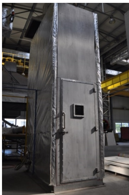
Figure 1. External view of EN 50399 standard test chamber at the accredited ITB Fire Testing Laboratory in Pionki, Poland.
