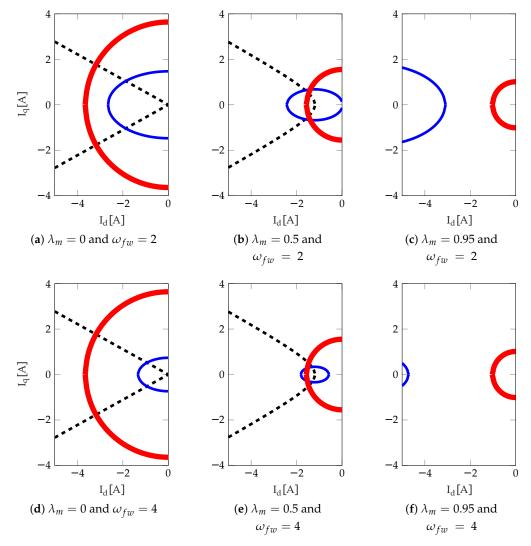
**Figure 4.** Voltage, current limits and MTPV curve at various PM flux  $\lambda_m$  and speed  $\omega$ .
