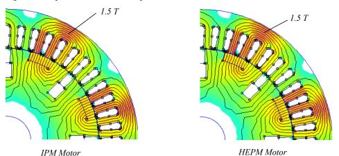
Figure 8. IPM and HEPM motor flux-density in MTPA at 1500 rpm.
