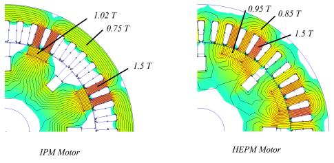
Figure 9. IPM and HEPM motor flux-density in FW at the end of FW operations.
