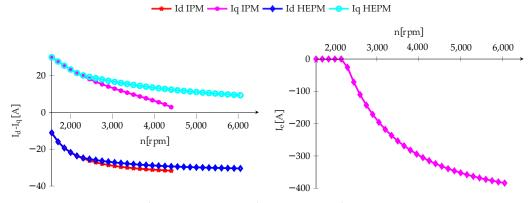
**Figure 6.** Rotor current and  $I_d - I_q$  in HEPM and IPM motors and Excitation current  $I_e$  in HEPM motor.
