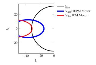
Figure 10. Voltage and current limits of HEPM and IPM at 4350 rpm.
