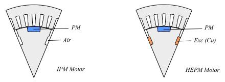
Figure 5. IPM and HEPM configuration.
