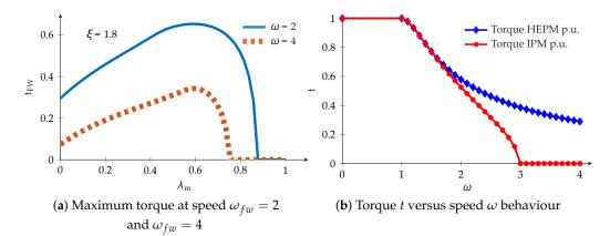
**Figure 3.** (a) Maximum torque that the motor can exhibit during Flux-Weakening (FW) operations according to the parameters and nominal current defined in Figure 2; (b) p.u. torque versus p.u. speed behaviors with and without the rotor flux reduction.
