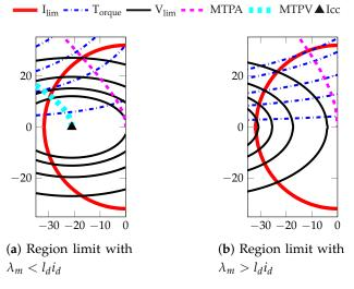
**Figure 1.** Operation area with an interior permanent magnet (IPM) motor with a high permanent magnet (PM) flux and low PM flux.
