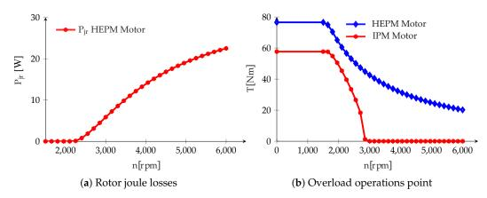
Figure 12. Rotor Joule losses and Torque with flux excitation in add to the PM flux.
