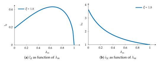
**Figure 2.** Normalized  $l_d$  and  $i_N$  versus rotor flux linkage ( $\lambda_m$  for IPM motor,  $\lambda_{HE,max}$  for HEPM motor) and  $\xi = 1.8$ .
