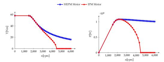
Figure 7. Torque and Power versus speed behaviors of the HEPM and IPM motors.
