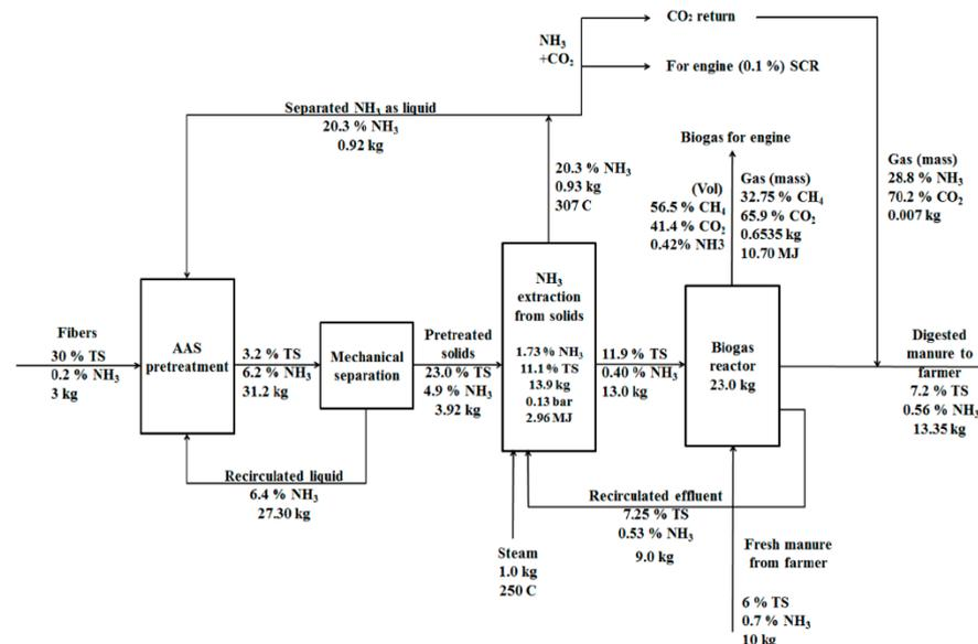
**Figure 2.** AD process of swine manure coupled with AAS pretreatment of manure fibers and  $\text{NH}_3$  recovery. All mass and energy units are expressed per hour.
