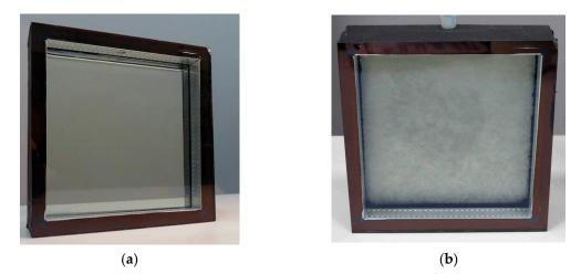
**Figure 3.** Glass sample prepared for experiment, (**a**) PCM in a liquid state and (**b**) PCM in solid state. The first cavity is empty, the second cavity is filled with PCM.
