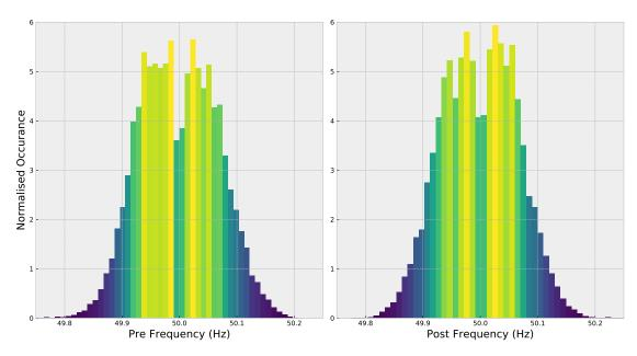
**Figure 8.** Comparison of pre- and post-action system frequency histograms. The plot on the left represents w/c 02/03/20 and the one on the right represents w/c 23/03/20. The post-action frequency distribution is concentrated more in the range of 49.9 to 50.1 Hz.
