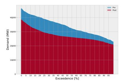
**Figure 4.** Load duration curve for pre- and post-lockdown actions (w/c 02/03/20 and 23/03/20) showing the decrease in the post-action scenario with the highest decrease in peak and lowest in the base load.
