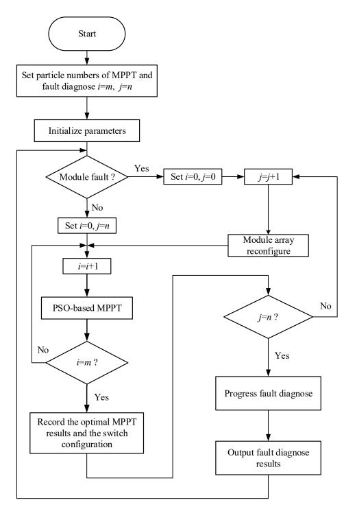
**Figure 3.** The step sequence of configuration optimization using particle swarm optimization (PSO) for a PV module array.
