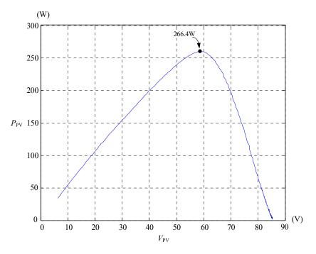
Figure 7. A single experimental P–V characteristic curve for all optimized configurations in Case 3.
