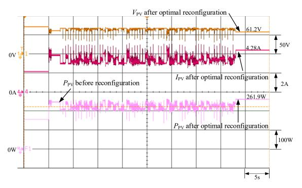
Figure 12. Response to an optimization request in a Case 1 array configuration.
