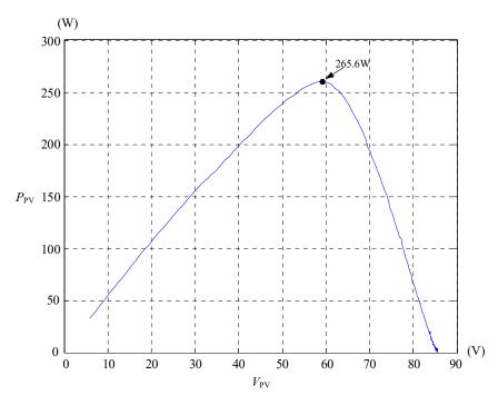
Figure 8. A single experimental P–V characteristic curve for all optimized configurations in Case 4.
