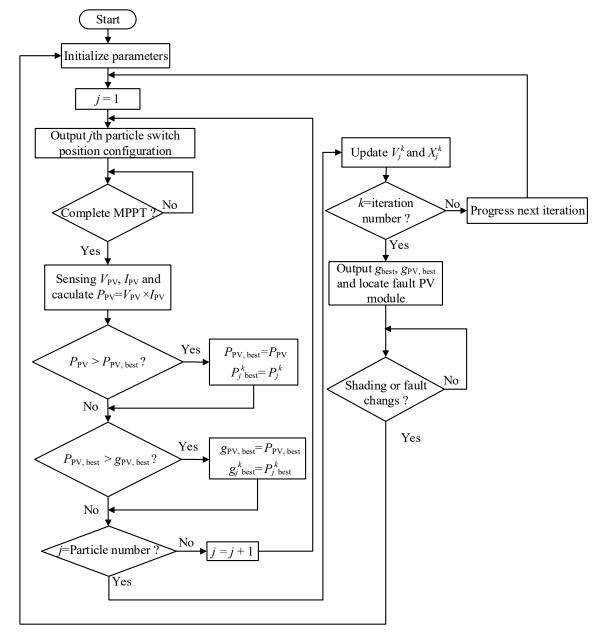
Figure 4. The flowchart of the configuration optimization using PSO for PV module array.
