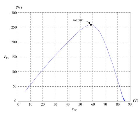
Figure 5. A single experimental P–V characteristic curve for all optimized configurations in Case 1.
