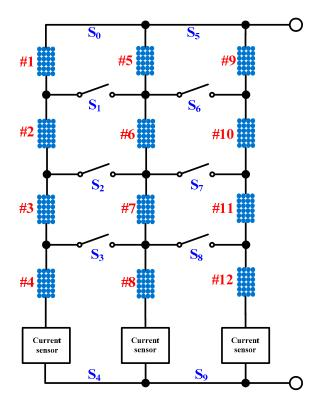
Figure 1. The presented photovoltaic (PV) module array configuration.
