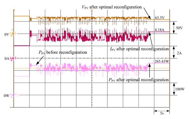
Figure 15. Response to an optimization request in a Case 4 array configuration.
