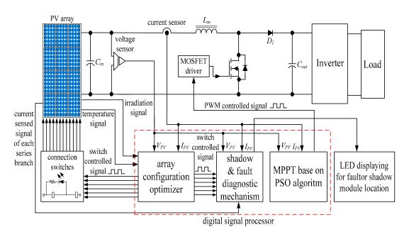
Figure 2. The framework of the presented online fault detection system.
