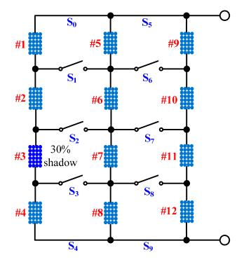
Figure 9. A pre-optimized array configuration with a 30% shadow in module 3.
