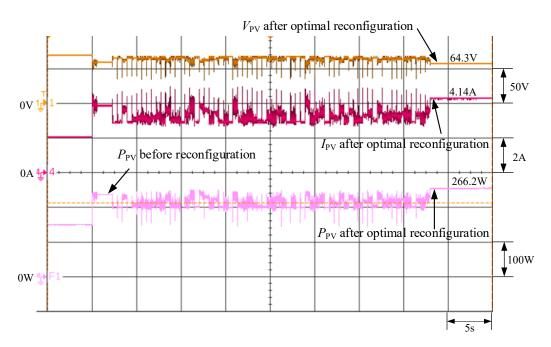
Figure 14. Response to an optimization request in a Case 3 array configuration.
