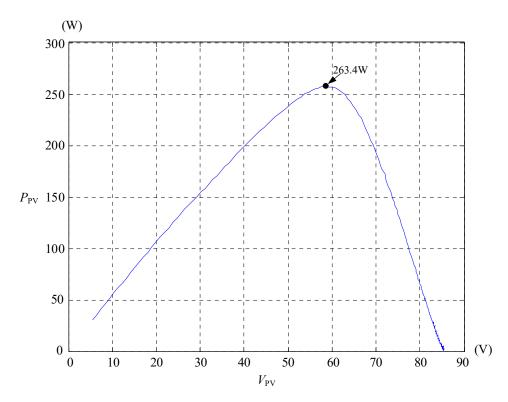
Figure 6. A single experimental P–V characteristic curve for all optimized configurations in Case 2.
