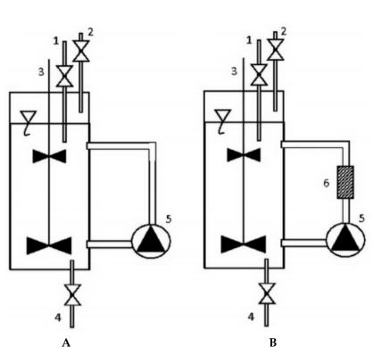
**Figure 1.** Design of the test site used for the experiments: (A—system without a magnetic fluid actuator (MFA), B—system with MFA, 1—substrate dosing, 2—biogas uptake, 3—vertical axis stirrer, 4—collection of the post-fermentation pulp, 5—circulating pump, 6—MFA).
