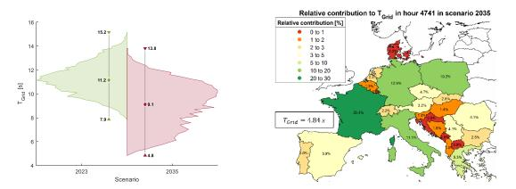
**Figure 14.** *T*<sub>grid</sub> for scenarios 2023 and 2035 (**left**) and each of the continental Europe (CE) region countries' contribution to system inertia for hour 4741 with lowest overall system inertia (**right**).
