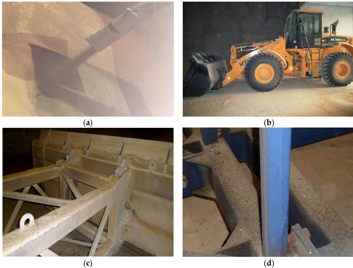
Figure 1. Examples of emission (a) and deposition of powdery fraction of seed meal on the floor of a warehouse (b) and machinery parts (c,d) (original photos by J. Chmiel, J. Halska).
