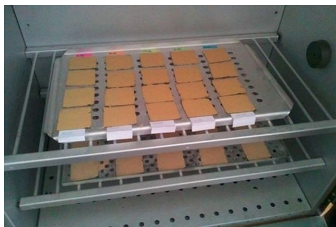
Figure 2. Specimens with a layer of biomass in a climate chamber.
