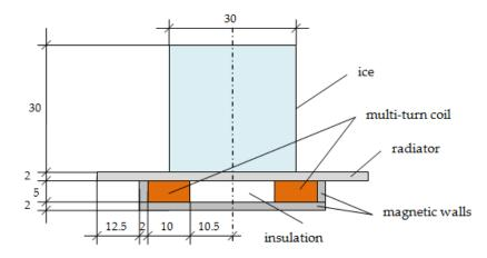
Figure 7. Geometry of IH coil with enclosure, radiator and ice on its surface (dimensions in millimeters).
