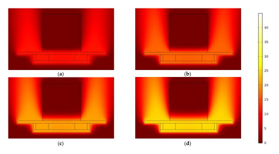
**Figure 11.** Temperature distribution (°C) around IH device (40 kHz, 2 A, 50 turns) for an initial temperature of 0 °C after 2 min (**a**), 4 min (**b**), 6 min (**c**), 8 min (**d**).
