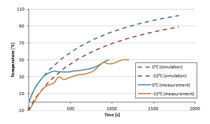
**Figure 12.** The temperature of the radiator surface vs. time for a frequency of 40 kHz and initial temperatures of 0 °C and -10 °C—simulation (solid lines) and measurement (dashed lines).
