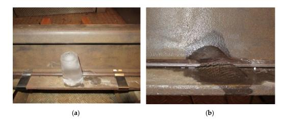
**Figure 5.** Ice piece melting with use of traditional resistive heating (RH) device: (**a**) initial stage; (**b**) partially melted ice.
