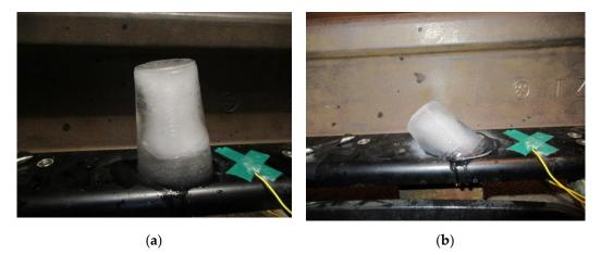
Figure 6. Ice piece melting with use of the IH device: (a) initial stage; (b) partially melted ice.
