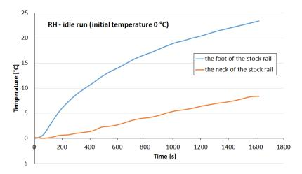
**Figure 13.** Foot and rail neck temperature vs. heating time in empty run of RH device for initial temperature 0 °C.
