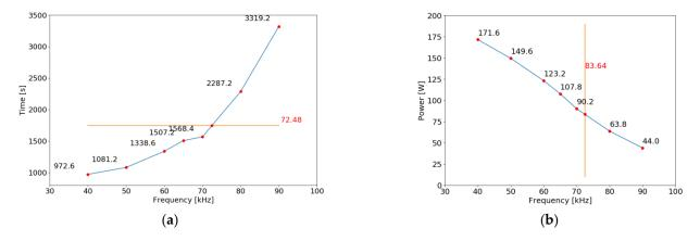
**Figure 17.** Determination of frequency and power used by a single RH device to melt ice piece at the same time as the RH device: (**a**) determination of frequency; (**b**) determination of power used.
