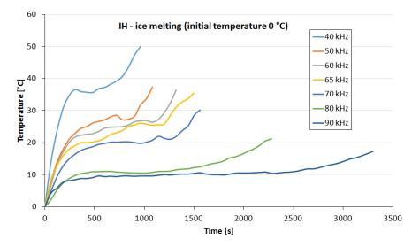
**Figure 15.** Temperature of IH device surface vs. time at different operating frequencies for an initial temperature of 0 °C.
