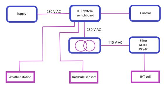
Figure 3. Elements of system for inductive heating of turnouts (IHT).
