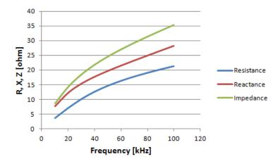
**Figure 9.** The resistance and reactance of the coil vs. frequency for 50 turns and assumed coil length 150 mm based on finite elements calculations.
