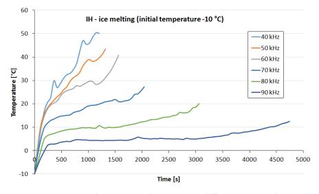
**Figure 16.** Temperature of IH device surface vs. time at different operating frequencies for an initial temperature of -10 °C.
