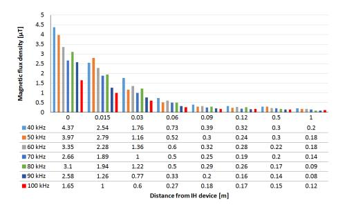
Figure 18. Magnetic flux density vs. distance from the IH radiator for various operating frequencies.
