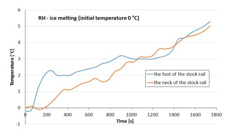
**Figure 14.** Foot and rail neck temperature vs. heating time during ice piece melting by RH device at an initial temperature of 0 °C.
