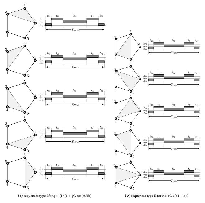
**Figure 8.** The switch state sequences in the basic solution of the gating signals for both converter cells  $CMC_P$  and  $CMC_N$ .
