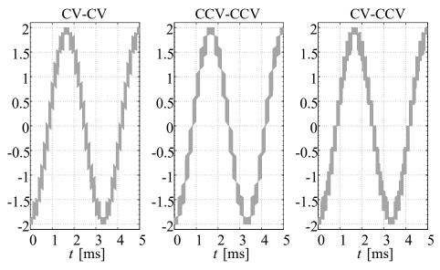
**Figure 12.** The load voltage  $v_0$  for DSM-CMC 12  $\times$  12 converter for the three selected modulation schemes:  $f_0 = 300$  Hz,  $q = 2 \times 0.95$ .
