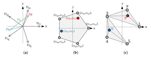
**Figure 6.** The principle of operation: (a) vectors arrangement, (b) synthesis field, and (c) selected triangles.
