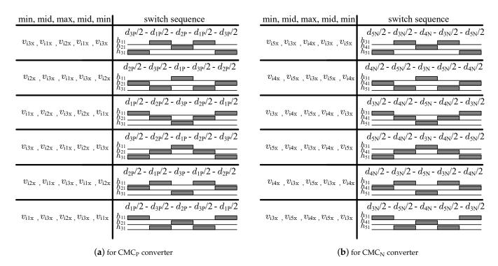
**Figure 9.** The MMM type of sequences of the gating signals for both converter cells  $CMC_P$  and  $CMC_N$  for the case depicted in Figure 6c.
