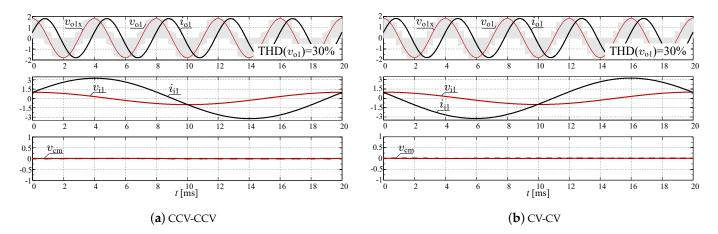
**Figure 17.** Simulation of the PWM variant 3 for DSM-CMC  $5 \times 5$  and two modulation schemes:  $f_0 = 250$  Hz, q = 1.8.
