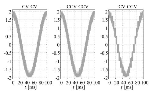
**Figure 11.** The load voltage  $v_0$  for DSM-CMC 12  $\times$  12 converter for the three selected modulation schemes:  $f_0 = 10$  Hz,  $q = 2 \times 0.95$ .
