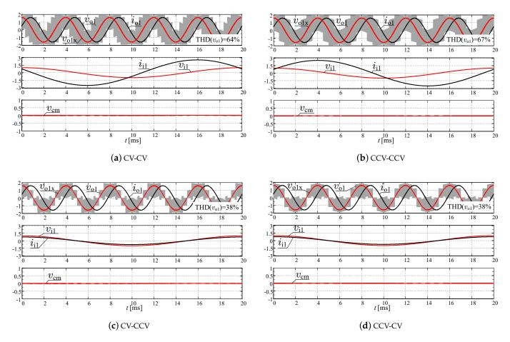
**Figure 10.** Simulation of the PWM variant 1 for DSM-CMC  $5 \times 5$  and four modulation schemes—RL load case.
