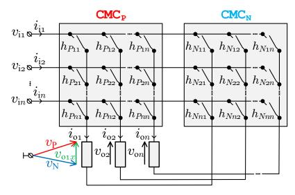
Figure 1. Simplified diagram of the square-type double conventional matrix converter.
