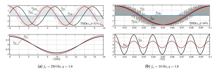
**Figure 18.** Simulation of the PWM variant 3 with toggling mode for DSM-CMC5  $\times$  5.
