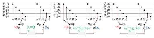
Figure 16. Sequences of the switch states in one commutation cell for the case presented in Figure 14.
