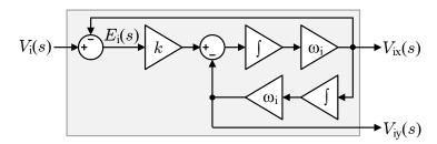
**Figure 4.** Double Second-Order Generalized Integrator with loop feedback extension functioned as Orthogonal Signal Generator (DSOGI-OSG) structure in continuous time-domain [33–35]:  $V_i$ —the input sinusoidal signal,  $V_{ix}$ —in-phase component of the input signal,  $V_{iy}$ —the quadrature component of the input signal,  $E_i$  the error signal,  $E_i$ —the gain block,  $E_i$ —reference pulsation of the input signal, and  $E_i$  is an integrator block.
