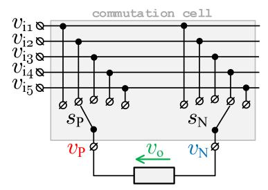
**Figure 2.** The single commutation cell for DSM-CMC  $5 \times 5$ .
