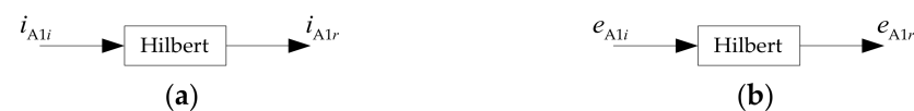
Figure 7. The orthogonal signals of the current and permanent magnet back EMF: (a) current signal; (b) back EMF signal.
