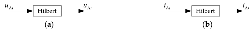
Figure 6. The orthogonal signal of phase A obtained by Hilbert transform: (a) Voltage signal of phase A; (b) current signal of phase A.
