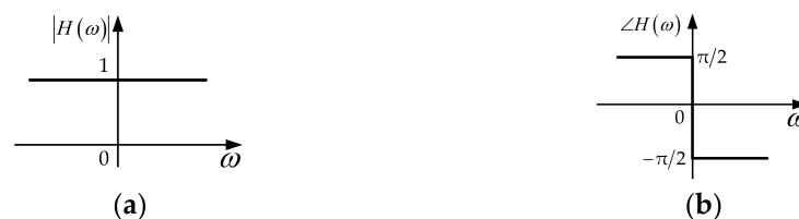
Figure 5. Amplitude–frequency and phase–frequency characteristics of Hilbert transform: (a) amplitude–frequency characteristics; (b) phase–frequency characteristics.
