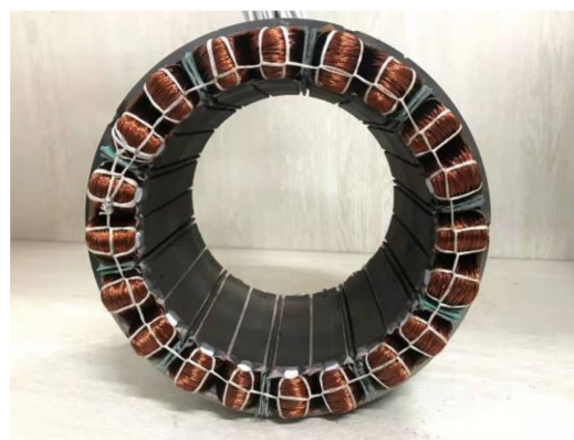
Figure 20. Stator winding structure of the five-phase PMSM.
