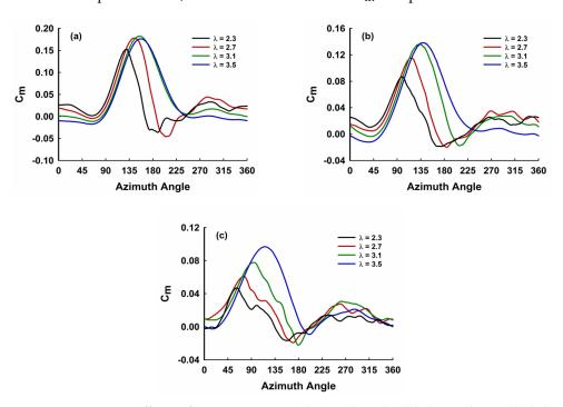
**Figure 8.** Moment coefficient for various tip speed ratios (TSRs), (a) helix angle  $60^{\circ}$ , (b) helix angle  $90^{\circ}$ , (c) helix angle  $120^{\circ}$ .
