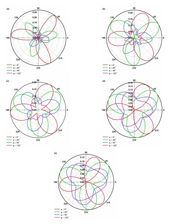
**Figure 12.** Cumulative polar plot of  $C_m$  comparing different helix angles and a straight blade at (a) TSR = 2.3, (b) TSR = 2.5, (c) TSR = 3.1, (d) TSR = 3.5, (e) TSR = 3.9.
