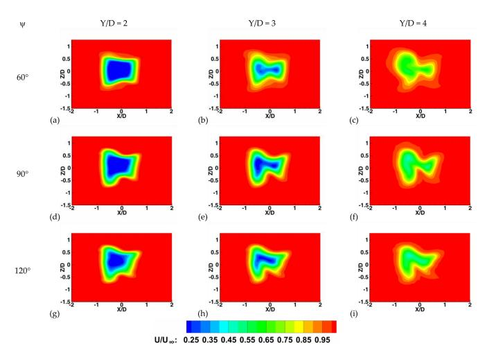
**Figure 23.** Wake structure of helical blade VAWT at Y/D of 2 ( $\mathbf{a}$ , $\mathbf{d}$ , $\mathbf{g}$ ), 3 ( $\mathbf{b}$ , $\mathbf{e}$ , $\mathbf{h}$ ), and 4 ( $\mathbf{c}$ , $\mathbf{f}$ , $\mathbf{i}$ ). For helical-bladed VAWT at TSR = 3.5.
