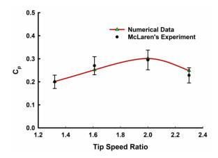
Figure 6. Validation of numerical results to McLarens experimental results.
