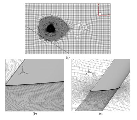
**Figure 3.** (a) Sectional view of the domain mesh: (b) mesh near the blade, (c) mesh growth surrounding the blade.
