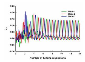
**Figure 5.** Cyclic convergence of solution for a  $60^{\circ}$  helical blade VAWT running at  $\lambda = 2.3$ .
