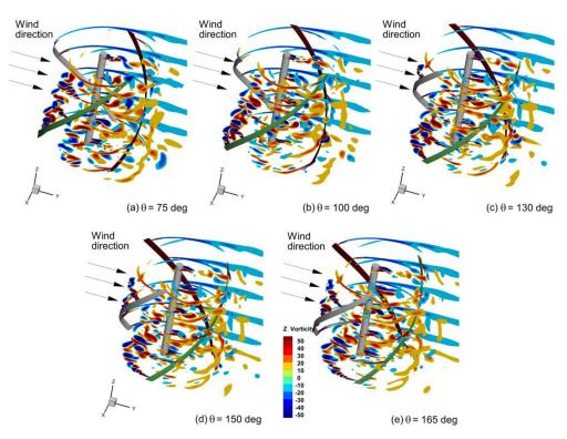
**Figure 19.** Z-vortex magnitude for 120° helical VAWT at z planes at heights of -1.45 m, -0.75 m, 0 m, 0.75 m, and 1.45 m at azimuth angles of rotation of (a)  $75^{\circ}$ , (b)  $100^{\circ}$ , (c)  $135^{\circ}$ , (d)  $150^{\circ}$ , and (e)  $165^{\circ}$ .
