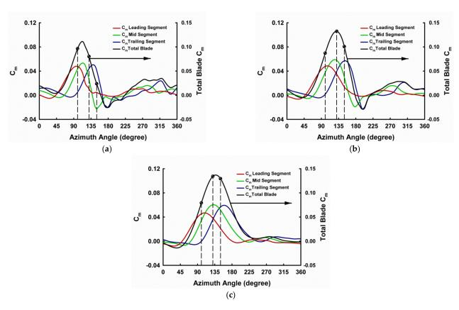
**Figure 20.** Section-wise  $C_m$  contribution of different segments of a single blade of a 90° helical VAWT operating at TSRs of (a) 2.7, (b) 3.1, and (c) 3.5.
