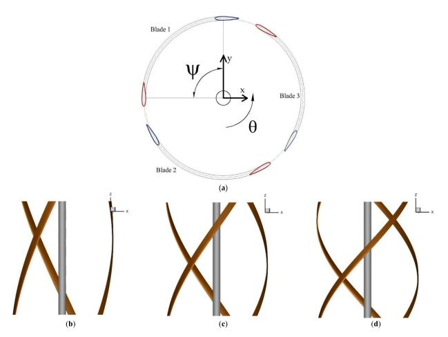
**Figure 1.** Top view of (a) Helical blade vertical axis wind turbines (VAWT) with definition of direction of rotation ( $\theta$ ) and helix angle ( $\psi$ ); front view of helical blade VAWT (b)  $\psi = 60^{\circ}$  (c)  $\psi = 90^{\circ}$  (d)  $\psi = 120^{\circ}$ .
