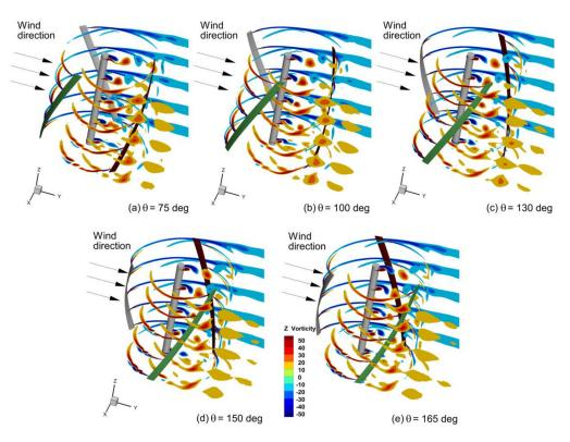
**Figure 17.** Z-vortex magnitude for  $60^{\circ}$  helical VAWT at z planes at heights of -1.45 m, -0.75 m, 0 m, 0.75 m, and 1.45 m at azimuth angles of rotation of (a)  $75^{\circ}$ , (b)  $100^{\circ}$ , (c)  $135^{\circ}$ , (d)  $150^{\circ}$ , and (e)  $165^{\circ}$ .
