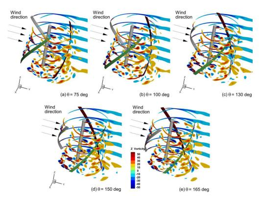
**Figure 18.** Z-vortex magnitude for  $90^{\circ}$  helical VAWT at z planes at heights of -1.45 m, -0.75 m, 0 m, 0.75 m, and 1.45 m at azimuth angles of rotation of (a)  $75^{\circ}$ , (b)  $100^{\circ}$ , (c)  $135^{\circ}$ , (d)  $150^{\circ}$ , and (e)  $165^{\circ}$ .
