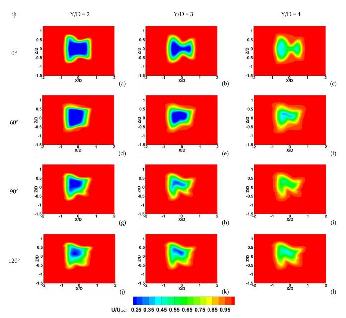
**Figure 22.** Wake structure of helical blade VAWT at Y/D of 2 (**a**,**d**,**g**,**j**), 3 (**b**,**e**,**h**,**k**), and 4 (**c**,**f**,**i**,**l**). For straight and helical-bladed VAWT at TSR = 3.1.
