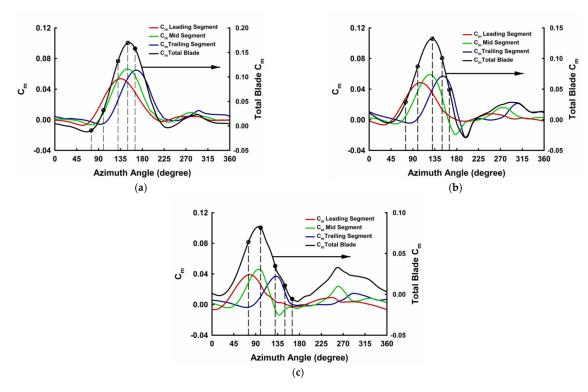
**Figure 16.** Section-wise  $C_m$  contribution of each segment of a single blade of (a)  $\phi = 60^\circ$ , (b)  $\phi = 90^\circ$ , and (c)  $\phi = 120^\circ$  helical-bladed VAWT operating at a TSR of 3.1.
