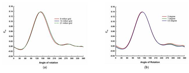
Figure 4. Moment coefficient (Cm) plot for a single blade indicating (a) grid independence, (b) time step independence.
