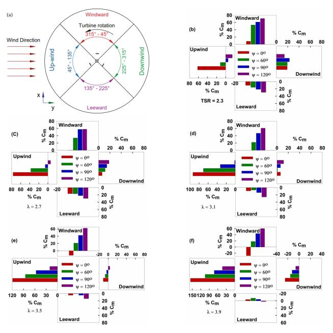
**Figure 13.** (a) Definition of quartile and percentage contribution by a blade in each quartile for all helical blades and straight blades at (b) TSR = 2.3, (c) TSR = 2.7, (d) TSR = 3.1, (e) TSR = 3.5, and (f) TSR = 3.9.
