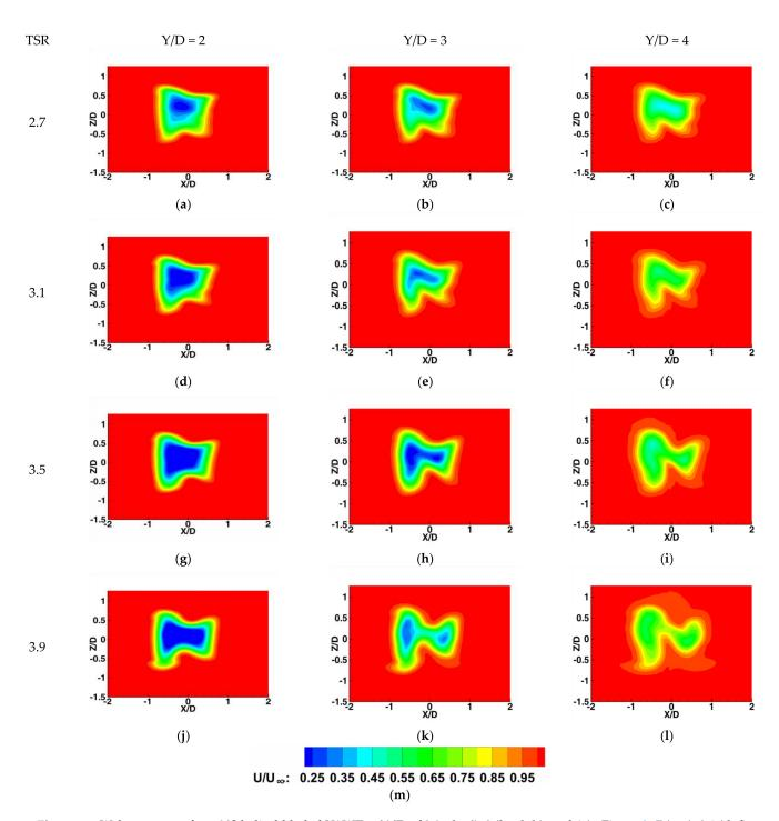
**Figure 24.** Wake structure for a 90° helical-bladed VAWT at Y/D of 2 ( $\mathbf{a}$ , $\mathbf{d}$ , $\mathbf{g}$ , $\mathbf{j}$ ), 3 ( $\mathbf{b}$ , $\mathbf{e}$ , $\mathbf{h}$ , $\mathbf{k}$ ), and 4 ( $\mathbf{c}$ , Figure 2. 7 ( $\mathbf{a}$ - $\mathbf{c}$ ), 3.1 ( $\mathbf{d}$ - $\mathbf{f}$ ), 3.5 ( $\mathbf{g}$ - $\mathbf{i}$ ) and 3.9 ( $\mathbf{j}$ - $\mathbf{l}$ ).
