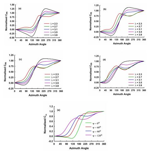
Figure 10. Normalised cumulative  $C_m$  Curve of blade 1 at different  $\lambda$  for (a)  $\psi = 0^\circ$ , (b)  $\psi = 60^\circ$  (c)  $\psi = 90^\circ$ , (d)  $\psi = 120^\circ$ , (e) Normalised curve of all helical-bladed turbines compared against straight blade turbine at a TSR of 3.1.
