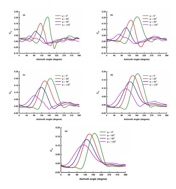
**Figure 9.** C<sub>m</sub> curve for the first blade of straight  $60^{\circ}$ ,  $90^{\circ}$ , and  $120^{\circ}$  helix angles of blades compared at (**a**)  $\lambda = 2.3$ , (**b**)  $\lambda = 2.7$ , (**c**)  $\lambda = 3.1$ , (**d**)  $\lambda = 3.5$ , and (**e**)  $\lambda = 3.9$ .
