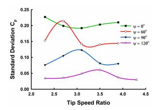
**Figure 14.** The standard deviation of C<sub>p</sub> of different helical-bladed and straight-bladed VAWT operating at different TSR.
