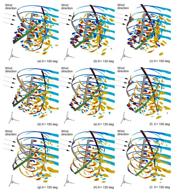
**Figure 21.** Z-vorticity magnitude of  $90^{\circ}$  helical-bladed VAWT at  $100^{\circ}$ ,  $130^{\circ}$ , and  $150^{\circ}$  of azimuth angles of rotation of a turbine operating at (a–c) TSR = 2.7, (d–f) TSR = 3.1, and (g–i) TSR = 3.5.
