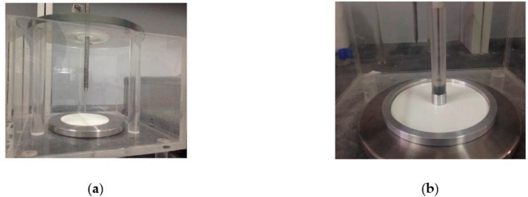
Figure 3. (a) Needle-plate electrode designed for a normal electric field (the length of the needle was 15 mm, the curvature radius of the tip was about 10\ \mu\text{m} and the gap distance was kept at 50 mm); (b) cylinder-annulus electrode designed for a tangential electric field (the inner electrode placed at the center was cylindrical with a diameter of 10 mm and height of 10 mm, the outer electrode was annulus with a height of 5 mm, external diameter of 110 mm and inner diameter of 100 mm, which was the same as the size of the sample).
