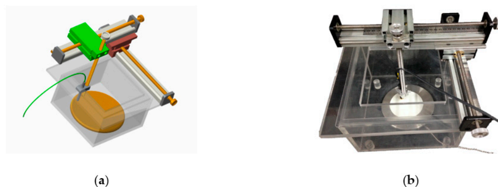
Figure 2. Surface potential measurement setup: (a) schematic diagram; (b) photo of the system.
