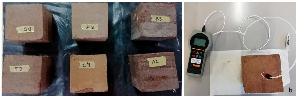
Figure 1. (a) Rammed earth samples; (b) Thermal conductivity measurements.
