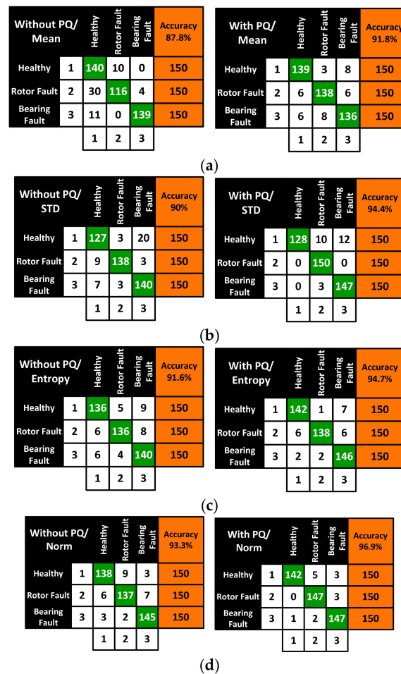
Figure 9. Confusion matrix of testing data with and without power quality for (a) mean, (b) standard deviation, (c) entropy, and (d) norm.
