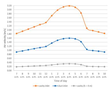
**Figure 6.** Hourly air velocity values referred to: duct inlet section, cavity inlet section (at the bottom of the façade), cross section of the cavity at a height of 4 m.
