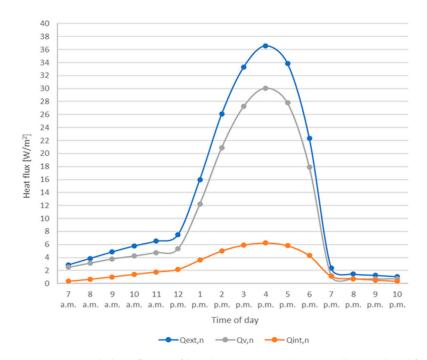
**Figure 8.** Hourly heat flux profiles obtained using the naturally ventilated façade:  $Q_{ext,n}$  is the heat flux coming from the external environment into the cavity,  $Q_{v,n}$  is the one removed by ventilation, and  $Q_{int,n}$  is the heat flux that flows from the cavity to the internal environment.
