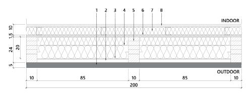
**Figure 1.** Horizontal section of the opaque ventilated façade module analyzed. The layers numbering refers to Table A1.
