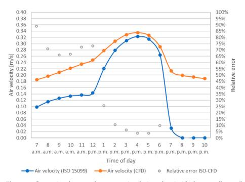
**Figure 12.** Comparison between the average air velocity values inside the naturally ventilated cavity calculated according to ISO 15099 and provided by the CFD simulations. The graph shows also the RE of the CFD compared to the standard, calculated until 6:00 p.m.
