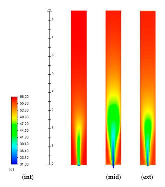
**Figure 15.** Temperature profile inside the naturally ventilated cavity at 4:00 p.m., plotted on the internal (**int**) and external (**ext**) surfaces of the cavity and on another surface (**mid**) at half its thickness.
