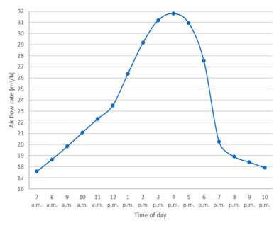
Figure 7. Hourly air flow rate through the naturally ventilated cavity.
