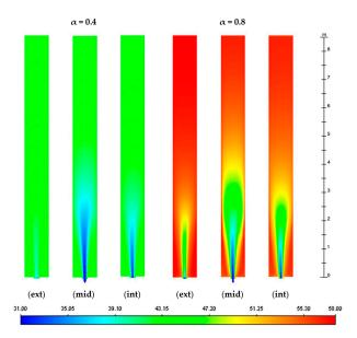
**Figure 16.** Comparison between the temperature profiles (indicated in  $^{\circ}$ C) at 4:00 p.m. on the external (ext) and internal (int) surfaces of the ventilated cavity and on a surface (mid) at half its thickness, considering  $\alpha = 0.4$  and  $\alpha = 0.8$ .
