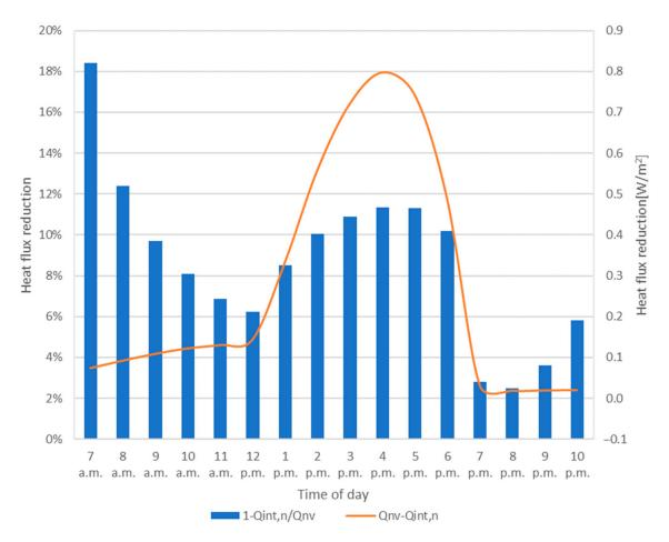
**Figure 18.** Hourly average energy saving  $(S_i)$  that could be reached using naturally ventilated façade instead of the unventilated one (the chart shows the average  $S_i$  values along the façade height).
