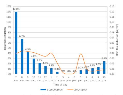
**Figure 9.** Hourly reduction of the heat flux entering the building provided by using forced ventilation  $(Q_{int,f})$  instead of natural ventilation  $(Q_{int,n})$ .
