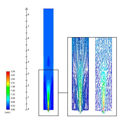
**Figure 14.** Air velocity profile inside the naturally ventilated cavity at 4:00 p.m., plotted on a surface at half the thickness of the cavity.
